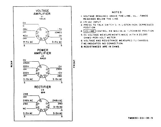
Figure 4. LS-147A/FI or LS-147B/FI, voltage and resistance chart.
