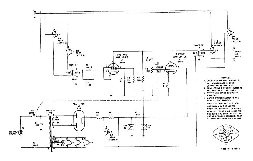
Figure 1. Intercommunication Station LS-147A/FI or LS-147B/FI, schematic diagram.
