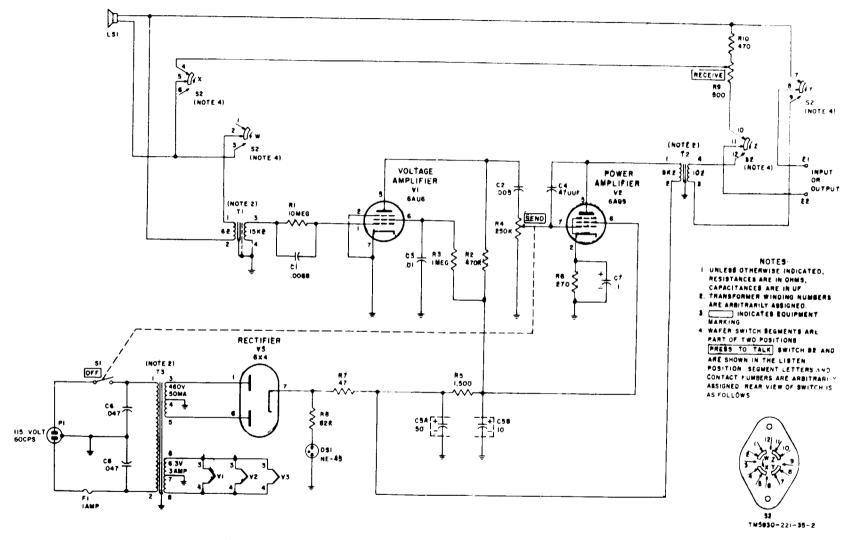
Figure 2. Intercommunication Station LS-147C/FI, schematic diagram.
