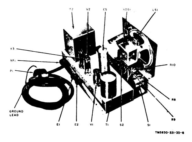
Figure 8. LS-147D/FI, less cabinet, top rear oblique view, location of parts.
