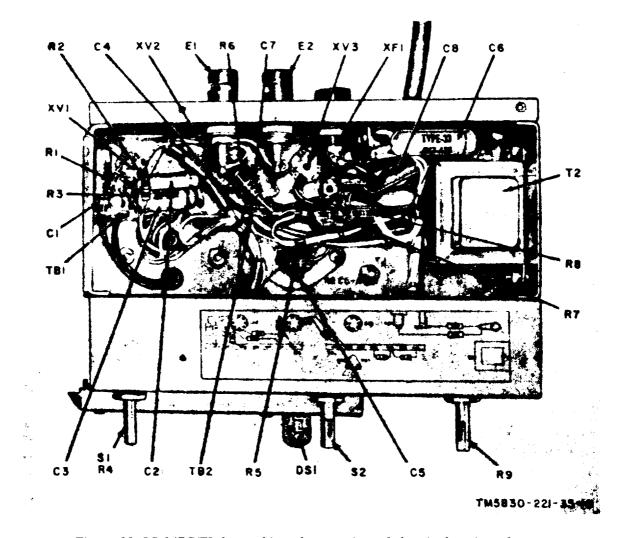
Figure 10. LS-147C/FI, less cabinet, bottom view of chassis, location of parts.
