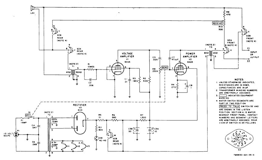
Figure 3. Intercommunication Station LS-147D/F1, schematic diagram.
