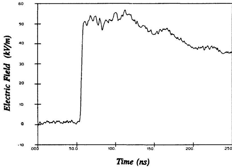
Figure B1: A typical Electric field wave form generated in the working volume of DREMPS.
