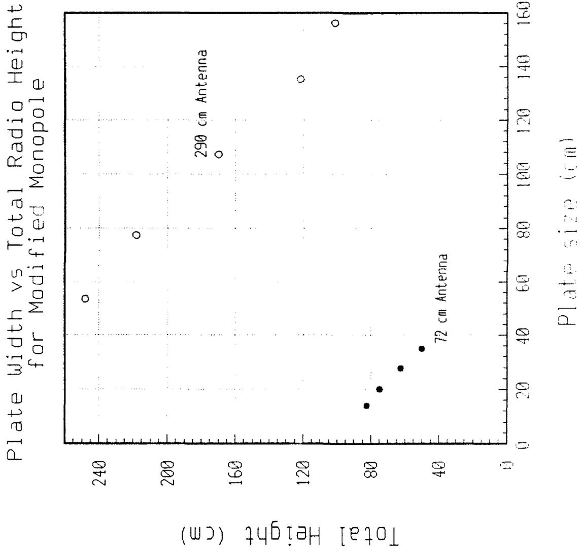
**Figure A2: A summary of the total radio (radio and antenna) height as a function of top plate diameter for the 72-cm and 290-cm antennae. Note that there is no reasonable plate substitution size for the latter.**
