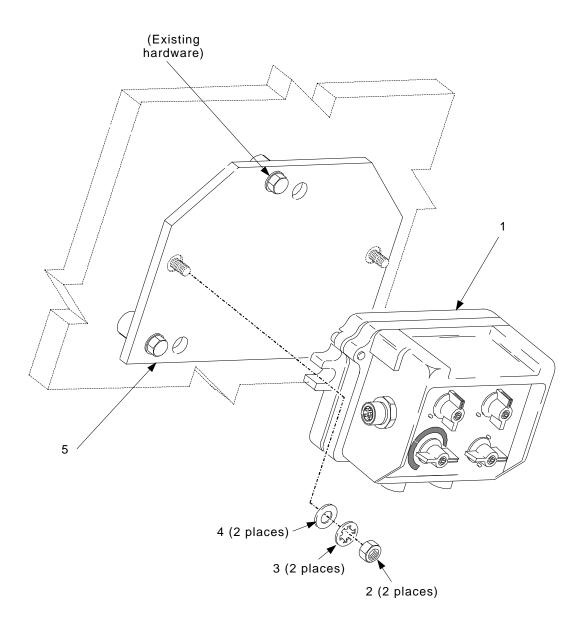
Figure 4-5. Gunner's FFCS Installation
