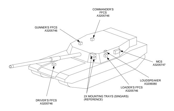
Figure 4-1. Equipment Location Diagram
