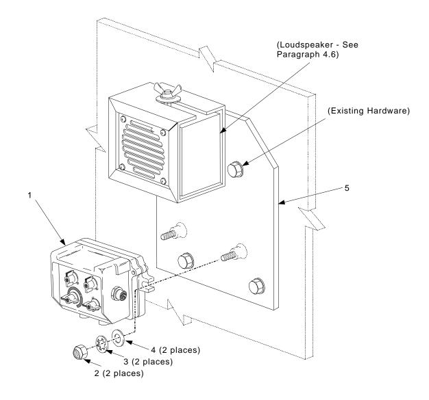
Figure 4-4. Loader's FFCS Installation
