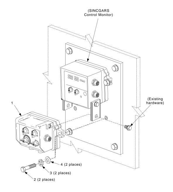
Figure 4-6. Commander's FFCS Installation
