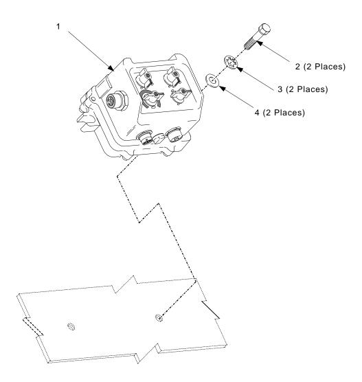
Figure 4-7. Driver's FFCS Installation
