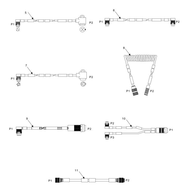
Figure 2-2. Illustrated Parts List - Cables
