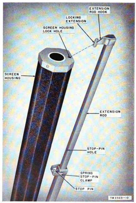
Figure 9. Screen PH-358-E, extension rod hook used to lock screen housing in vertical position.
