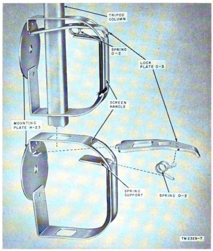
Figure 12. Screen PH-358-C, screen-handle assembly disassembled.
