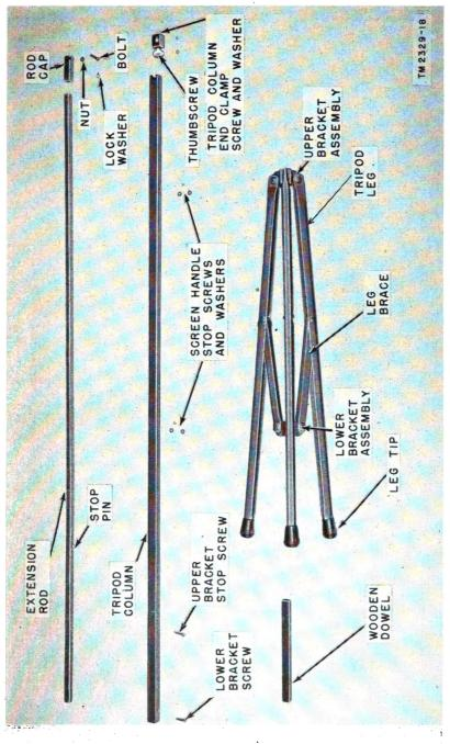
Figure 14. Screen PH-358-D, tripod assembly disassembled.
