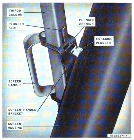
Figure 16. Screen PH-358-E, engaging plunger removed.
