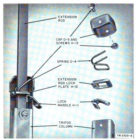
Figure 13. Screen PH-358-C, disassembly of extension rod lock assembly.
