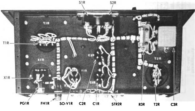
Figure 84. Remote Control Unit RM-45-A, bottom view.
