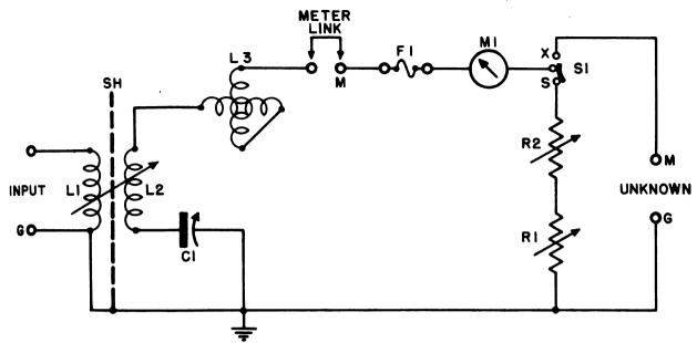
Figure 56. Impedance Measuring Box, circuit diagram.
