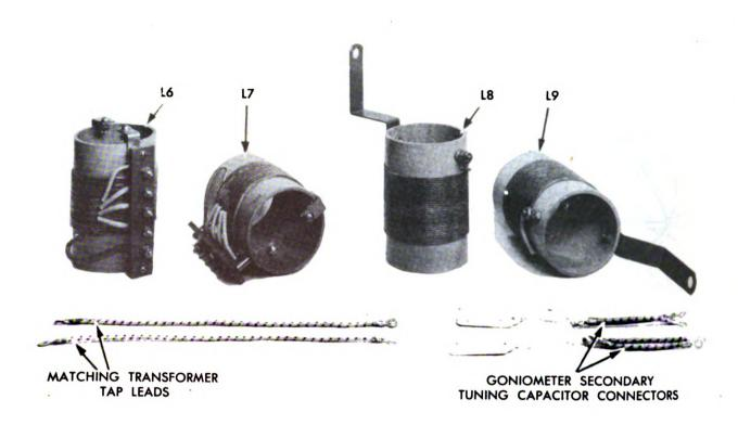
(Left background) goniometer primary matching transformers; (right background) goniometer secondary loading coils; (left foreground) matching transformer tap leads; (right foreground) goniometer secondary tuning caracitor banks paralleling connectors.
