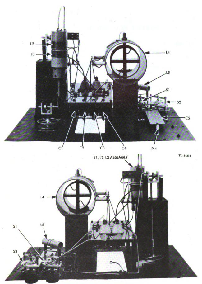
Figure 54. Antenna tuning unit, top and bottom views.
