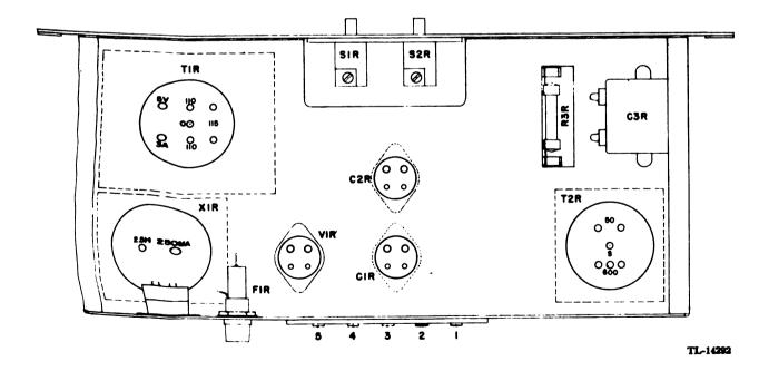
Figure 92. Remote Control Unit RM-45-A, chassis location diagram, bottom view.
