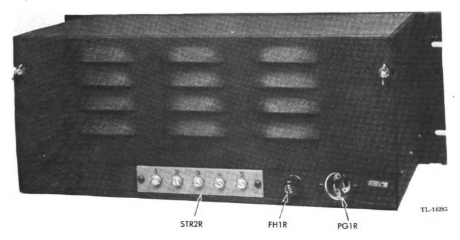
Figure 85. Remote Control Unit RM-45-A, rear view.
