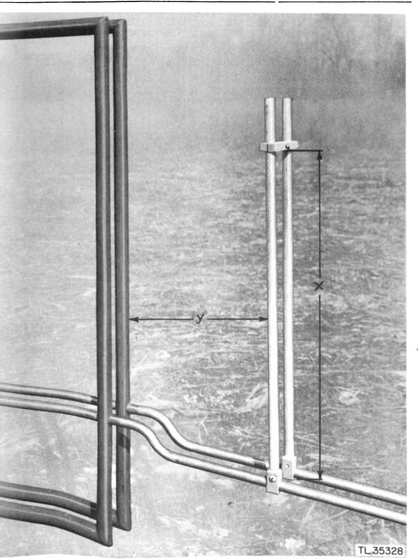
Figure 19. Antenna AN-161, antenna tuning stub.
