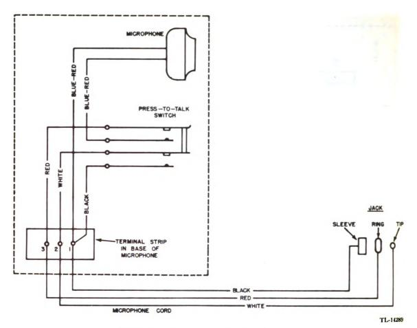
Figure 89. Microphone T-32, wiring diagram.
