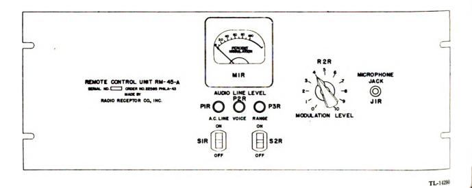
Figure 90. Remote Control Unit RM-45-A, front panel location diagram.
