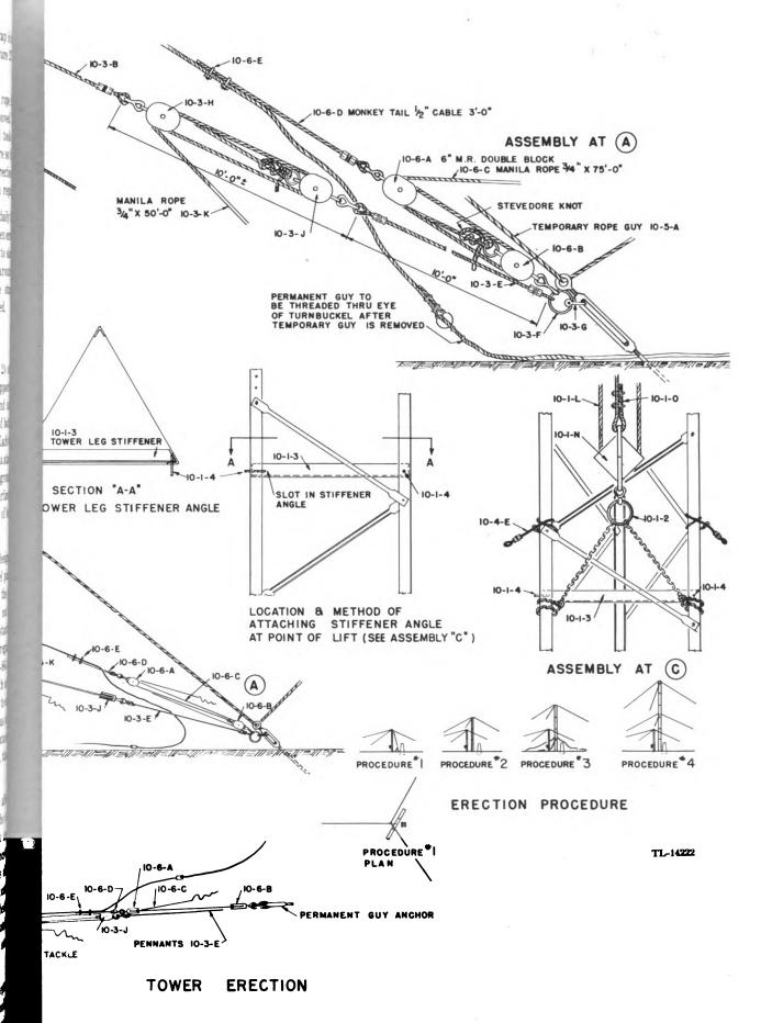
Figure 22. Tower erection details.
