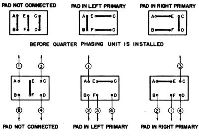
CONNECTIONS TO BE MADE WHEN INSTALLING QUARTER PHASING UNIT. NUMBERED LEADS SHOWN GO TO R.F. RELAY ON QUARTER PHASING UNIT. REFER TO FIGS. 70 AND 72 FOR CONNECTION OF LEADS 5 & 6
