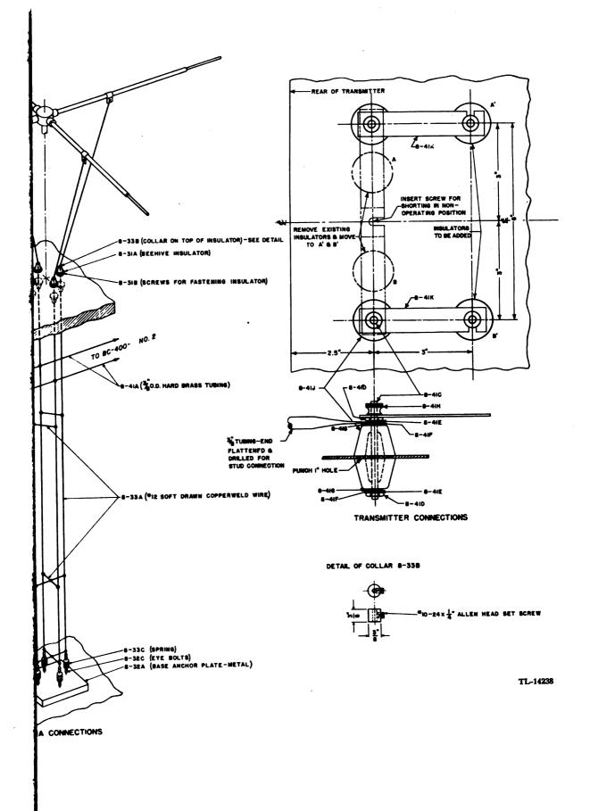
Figure 38. Marker antenna and marker antenna bus, details.
