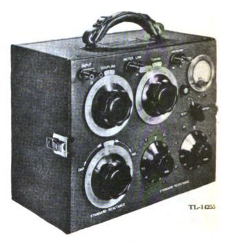
Figure 55. Impedance Measuring Box.
