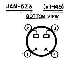
PIN I - FILAMENT PIN 2 - PLATE PIN 3 - PLATE PIN 4 - FILAMENT
