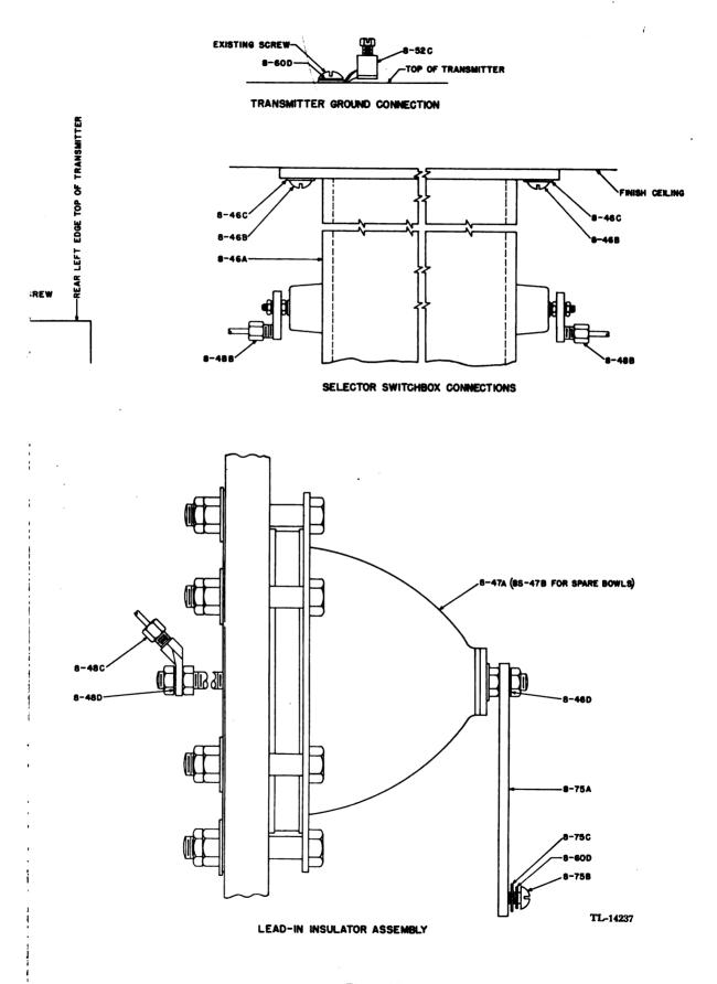
Figure 37. R-f bus mounting and connecting details for Radio Transmitter BC-446-(\*).
