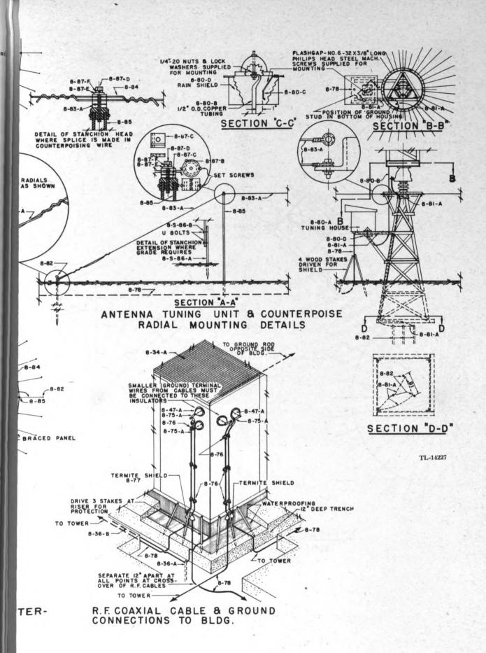
Figure 27. Antenna assembly, electrical cables.
