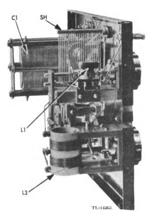
Figure 63. Impedance Measuring Box, left side interior view.
