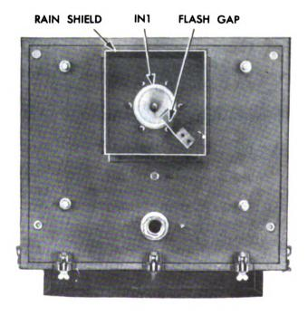
Figure 51. Antenna tuning unit, bottom view and transmitter tuning elements.
