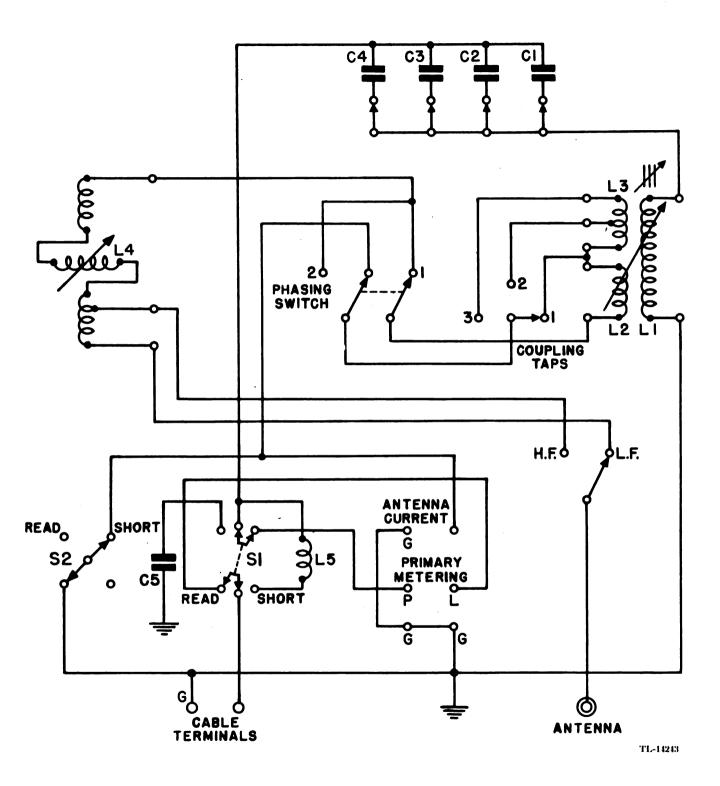
Figure 43. Antenna tuning unit, circuit diagram.
