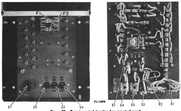
Figure 79. Remote control junction box, terminal panel cover removed, and rear view of panel.
