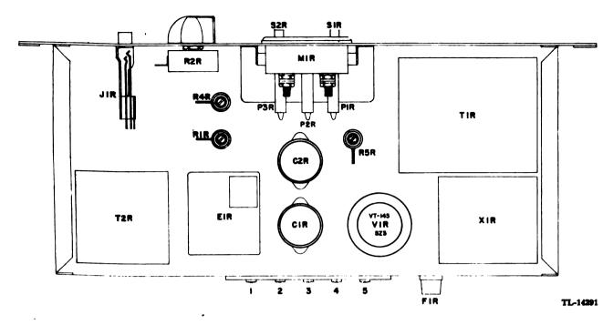
Figure 91. Remote Control Unit RM-45-A, chassis location diagram, top view.
