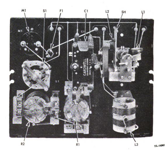
Figure 62. Impedance Measuring Box, rear interior view.
