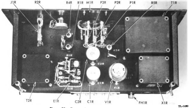
Figure 83. Remote Control Unit RM-45-A, interior view.
