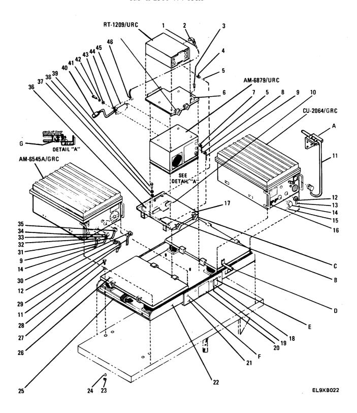
E-1 Installation Kit, Electronic Equipment, MK-2460/GRC-193A (Excluding Antenna Equipment Group 03) (Sheet 1 of 4)
