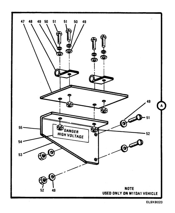
E-1 Installation Kit, Electronic Equipment, MK-2460/GRC-193A (Excluding Antenna Equipment Group 03) (Sheet 2 of 4)
