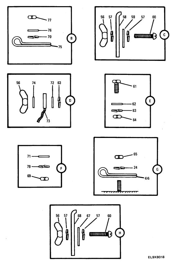
E-1 Installation Kit, Electronic Equipment, MK-2460/GRC-193A (Excluding Antenna Equipment Group 03) (Sheet 3 of 4)
