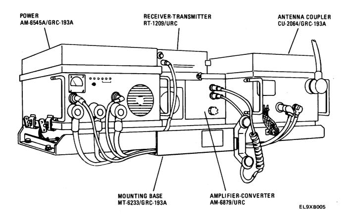
INSTALLATION KIT, ELECTRONIC EQUIPMENT MK-2460/GRC-193A
