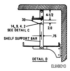
Drill two 7/32-inch holes in the shelf support bar using cable hanger assembly (item 30) as a template. Mount cable hanger assembly (item 30) using the #10 screws, nuts, lockwashers, and flat washers (items 14,9,4, and 2) provided. Cut and prepare antenna cable (item 22) as per detail B so that there is approximately 2 inches of slack in the cable.
