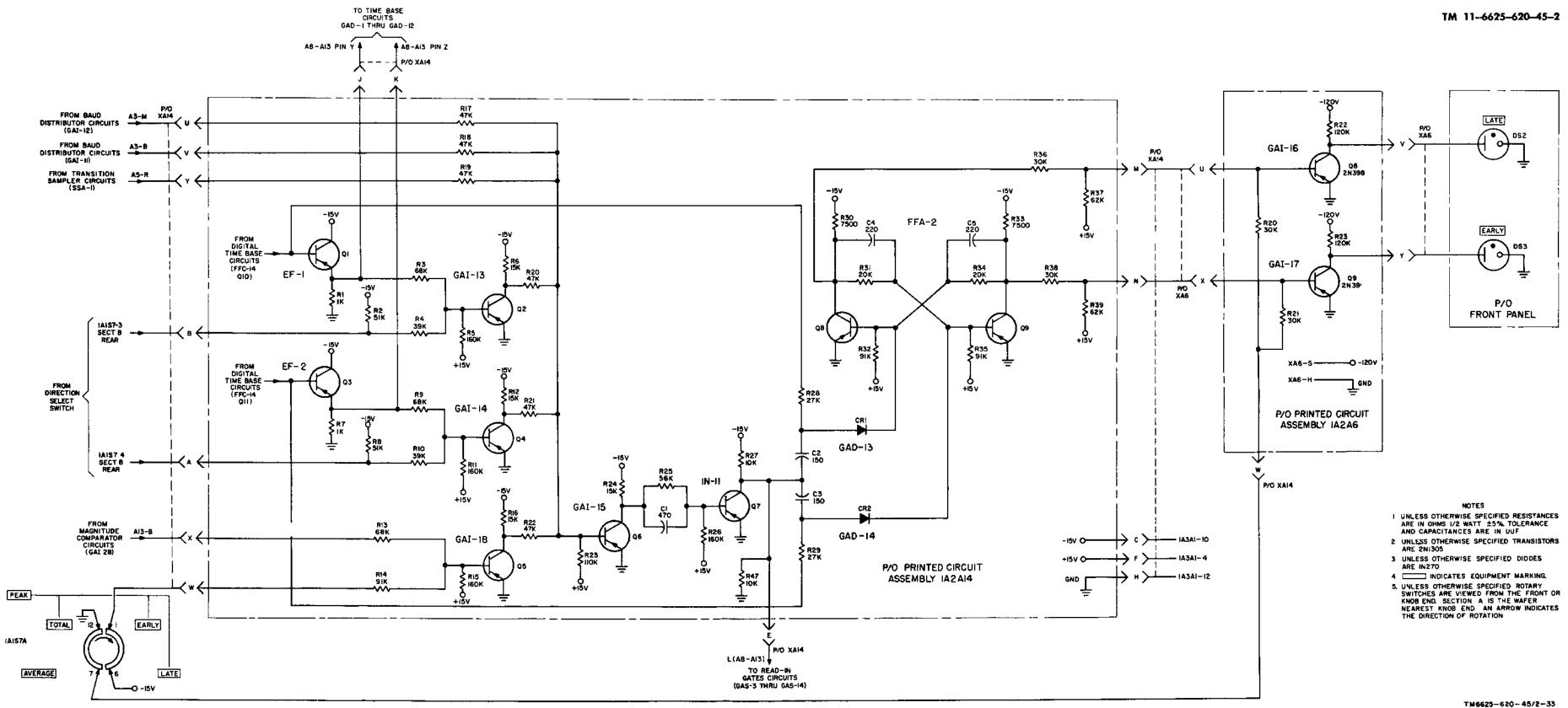
Figure 6-8. Sariy-late logic and transition-sampler control circuits, schematic diagram
