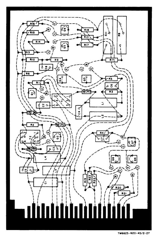
Figure 2-8. Printed circuit card assembly 1A2A6 (80047010), component locations.
