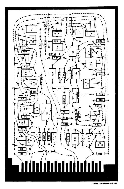
Figure 2-3. Printed circuit card assembly 1A2A1 (80047060), component locations.
