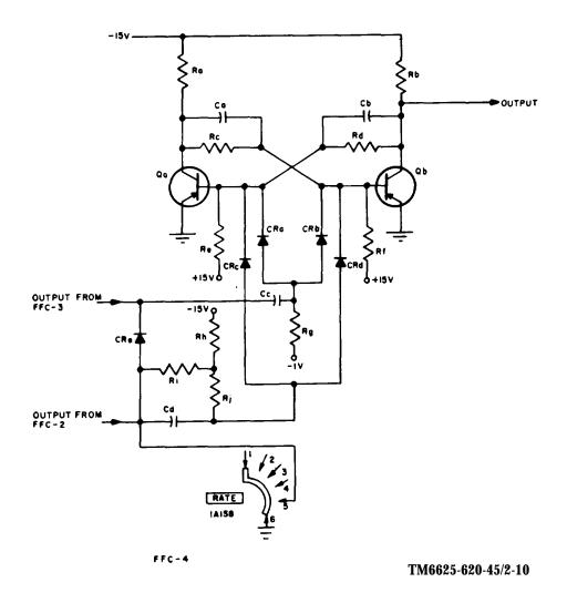
Figure 1-9. Time-base frequency-divider network
