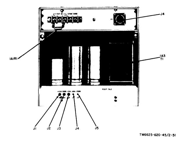
Figure 2-18. Rear view, component locations.
