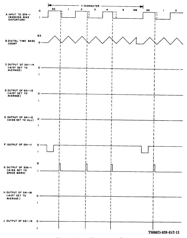
Figure 1-11. Average distortion, timing diagram.
