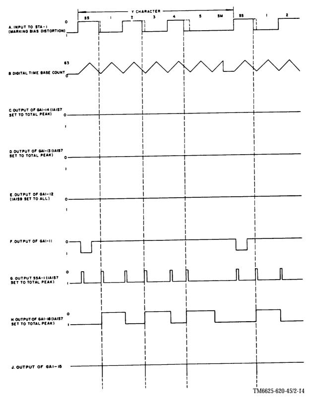
Figure 1-13. Early peak distortion, timing diagram.
