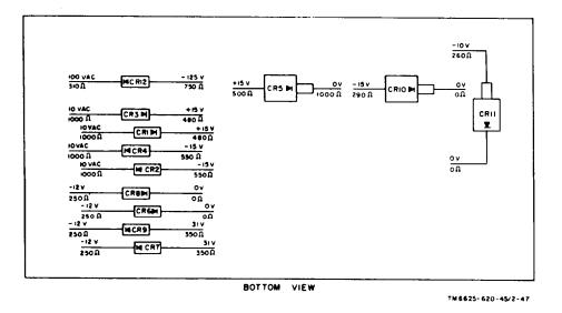
Figure 2-20. Printed circuit card assembly 1A3A1, voltage and resistance diagram.
