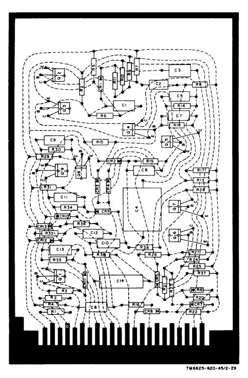
Figure 2-10. Printed circuit card assembly 1A2A8 (80047040), component locations.
