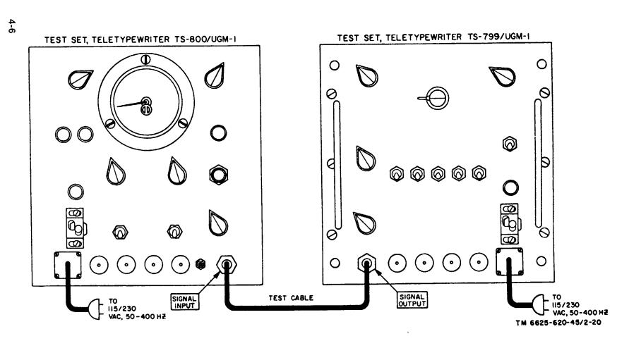
Figure 4-2. Distortion measurement test setup.
