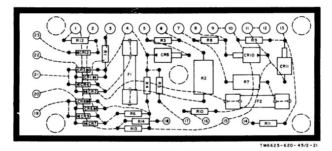
Figure 2-2. Printed circuit card assembly 1A3A1 (80047110), component locations.
