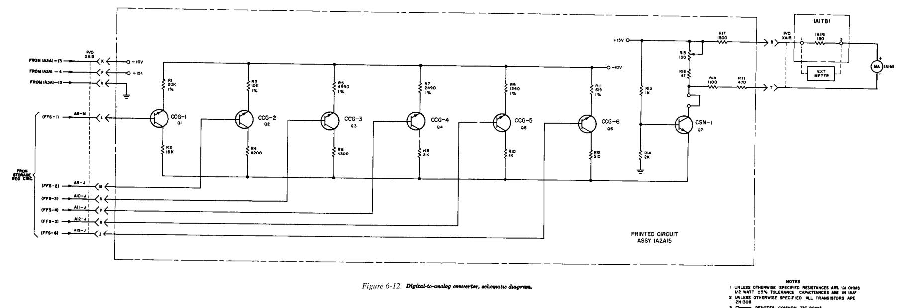
Figure 6-12. Digital-to-analog converter, schematro dragram.
