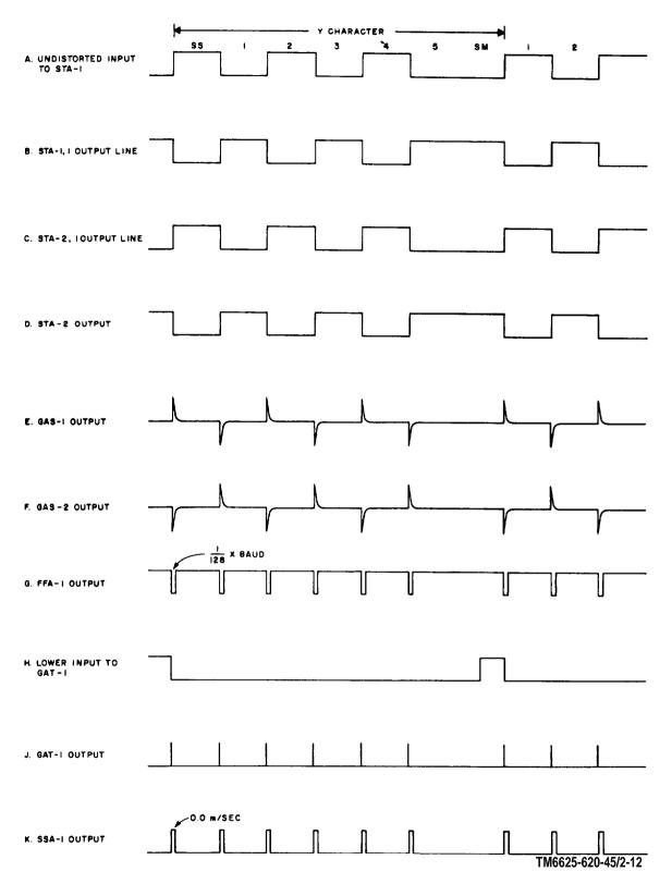
Figure 1-10. Transition sampler circuits, timing diagram.
