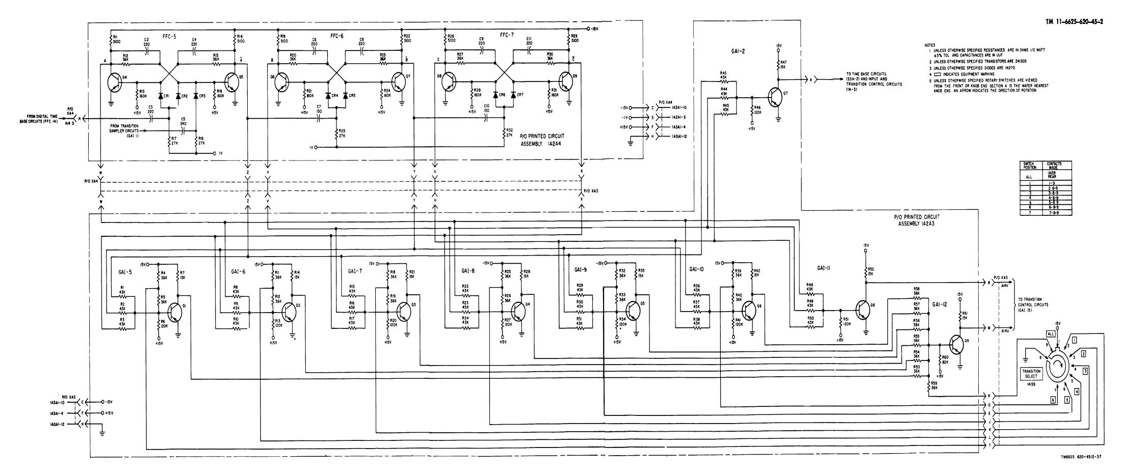
Figure 6-11. Baud distributor circuits, schematic diagram.
