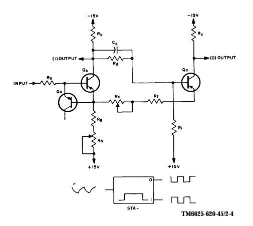
Figure 1-3. Schmitt trigger stage.
