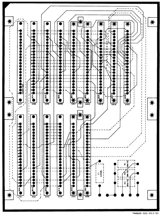
Figure 2-14. Harness board, component locations.
