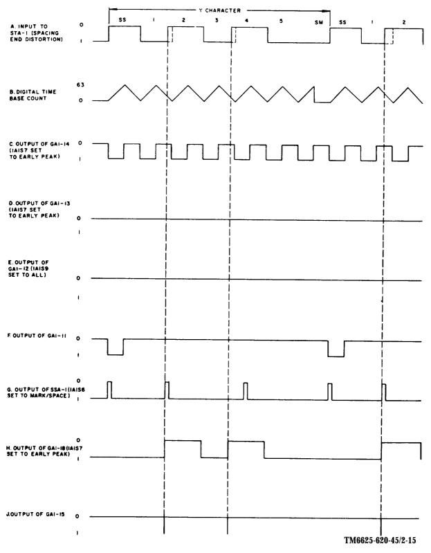
Figure 1-13. Early peak distortion timing diagram.
