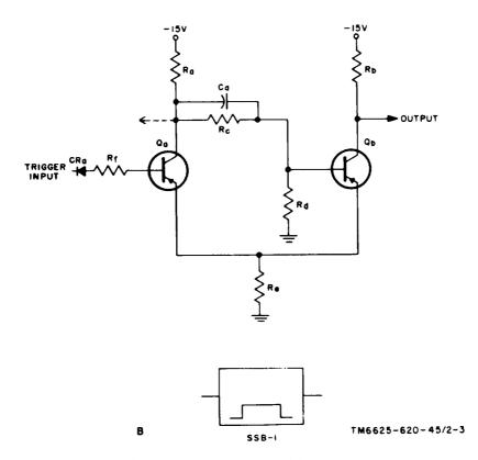
Figure 1-2. Monostable multivibrator stage.
