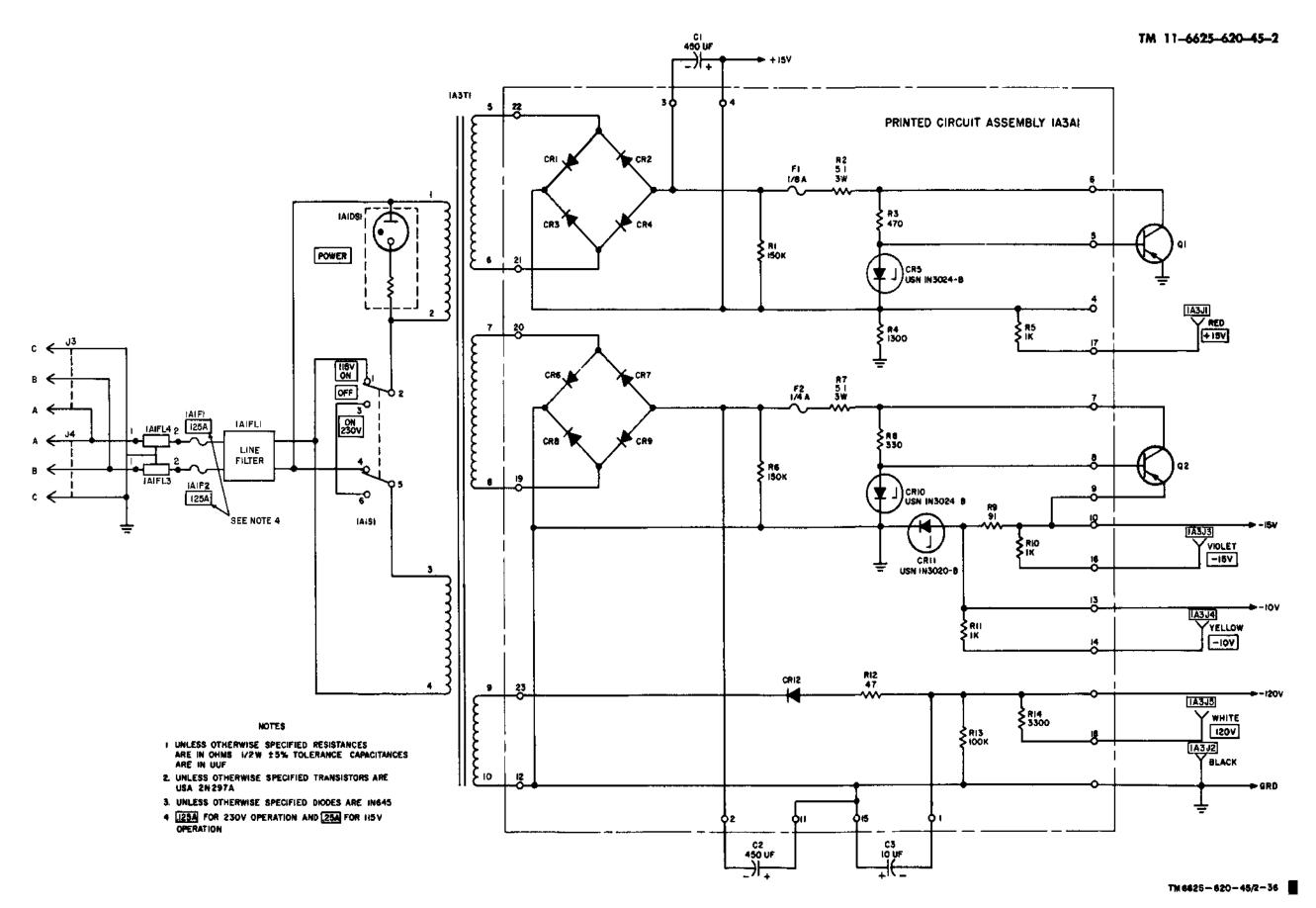
Figure 6-10. Power supply, schematic diagram.
