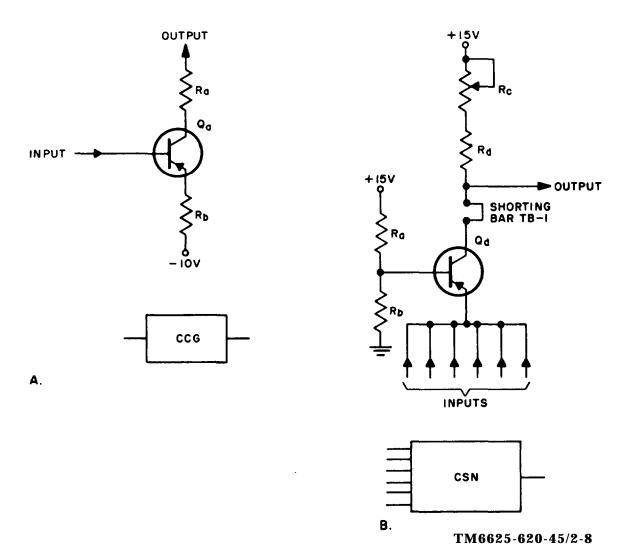
Figure 1-7. Constant-current genarator and summing stages.
