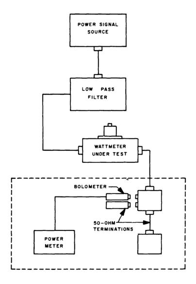
Figure 7-1. Coupler-Detector Test Set-up
