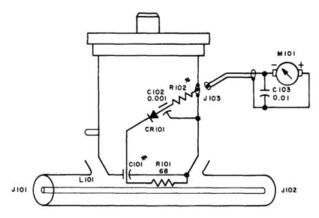
Figure 1-2. Wattmeter AN/URM-120, Schematic Diagram
