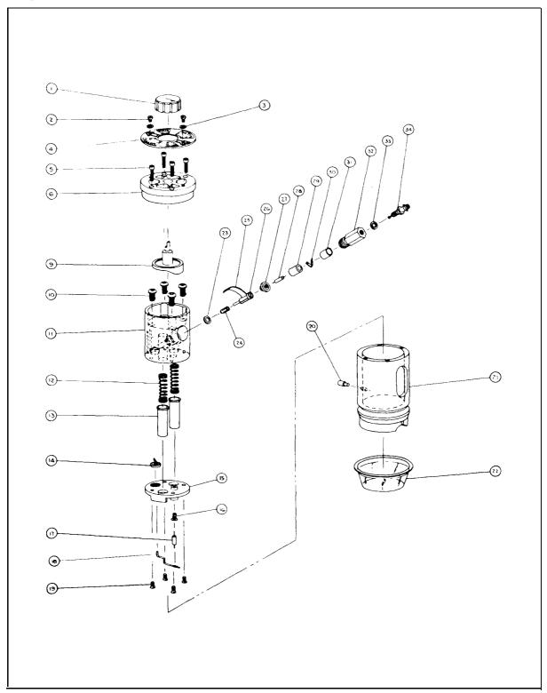
Figure 9-3. Coupler-Detector, Exploded View
