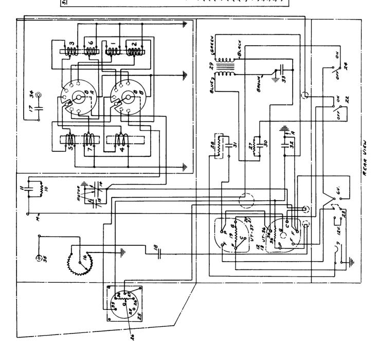
FIG.S. CONNECTION DIAGRAM OF OSCILLATOR TYPE BC-RC-183
