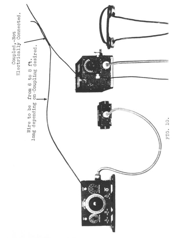
INSTALLATION AS OSCILLATOR EQUIPMENT, TYPE RC-12.
