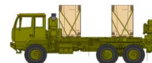
M1084 TRUCK CARGO: MTV W/MHE W/XM 501 GUIDED MISSILE SYSTEM SURFACE ATTACK (NLOS)
