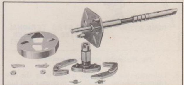
Fig. 38—Distributor Automatic Advance Mechanism
