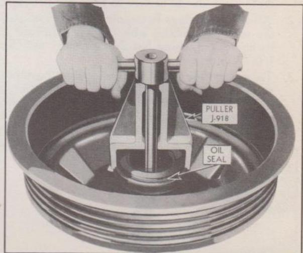
Fig. 16—Removing Inner Bearing and Oil Seal
