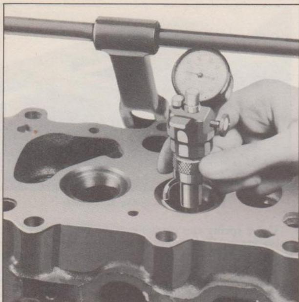
Fig. 49—Checking Valve Seat with Indicator Gauge
