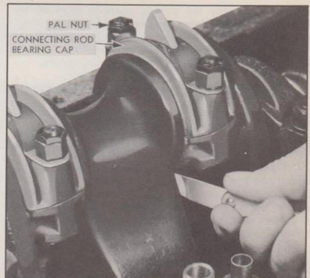
Fig. 34—Checking Connecting Rod Bearing Side Clearance
