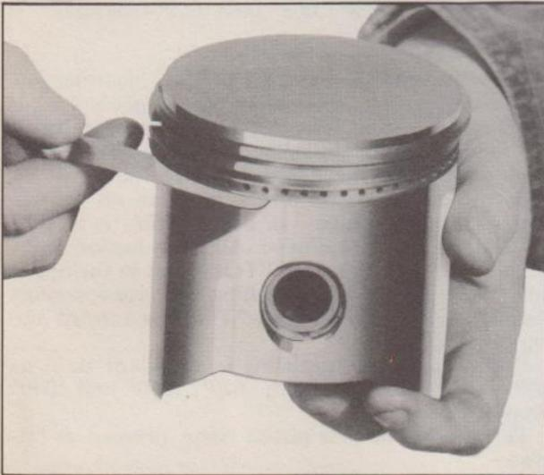
Fig. 7—Checking Piston Ring Clearance
