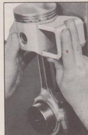
Fig. 31—Checking Piston and Connecting Rod Assembly
