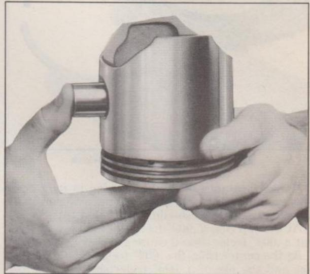
Fig. 5—Checking Piston Pin Fit
