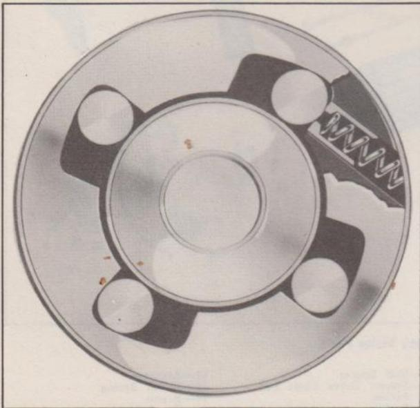
Fig. 33—Over-running Clutch
