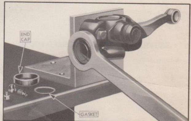
Fig. 11—Removing End Caps from Double-Acting Shock Absorbers
