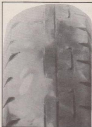
Fig. 5—Wear Due to Mechanical Condition
