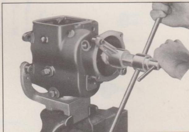
Fig. 5—Removing Mainshaft
