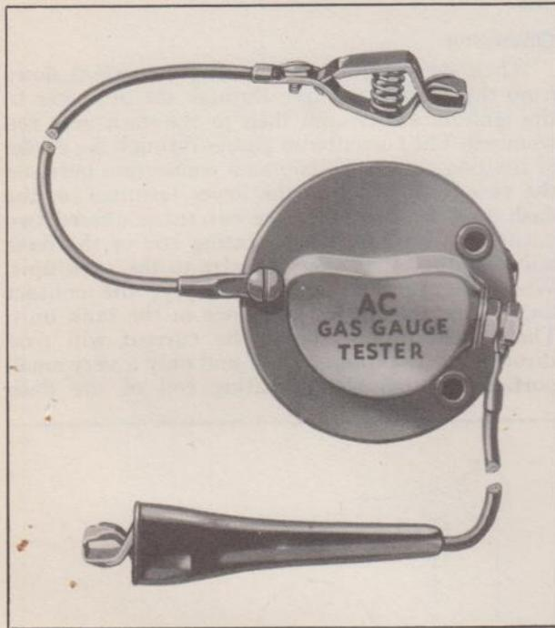
Fig. 46—Gasoline Gauge Tester
