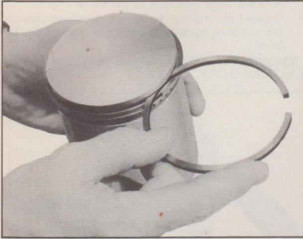
Fig. 6—Checking Ring Fit in Groove
