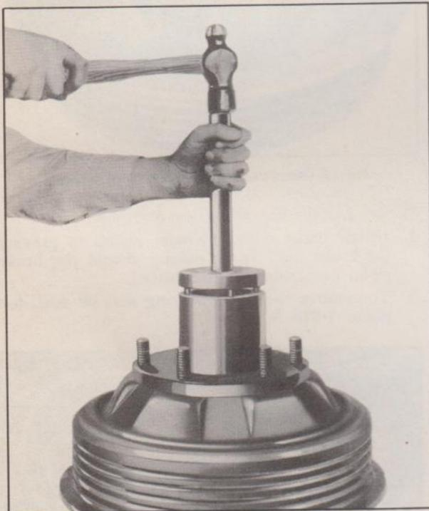
Fig. 18—Driving Outer Race into Contact with Snap Ring
