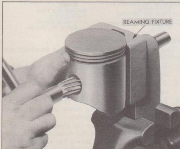
Fig. 4—Reaming Piston Pin Bushings
