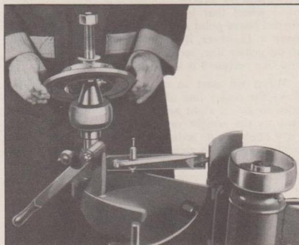
Fig. 9—Installing Leveling Plate
