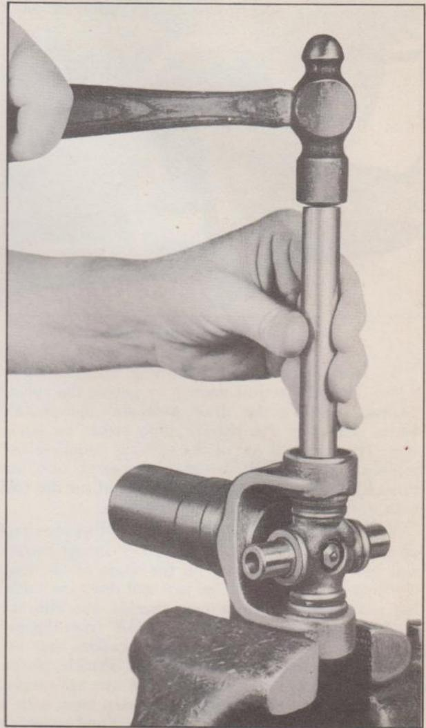
Fig. 42—Removing Trunnion Bearings from Joint Yoke
