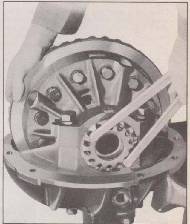
Fig. 28—Adjusting Ring Gear and Pinion Back Lash
