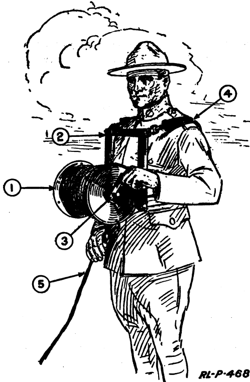
Fig. 1 - IG.—The breast reel, incorrectly slung
