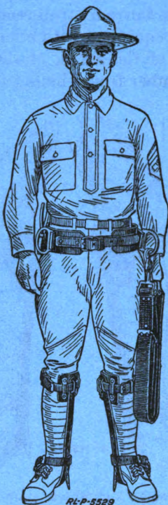
Fig. 2.—Lineman's equipment, properly adjusted
