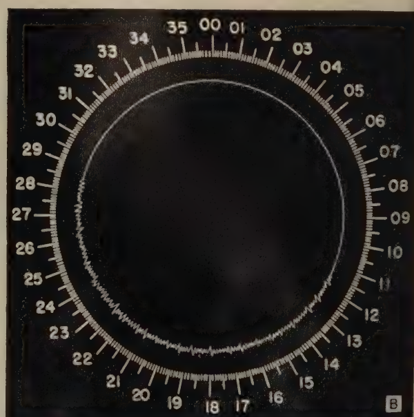
Figure 181. Indicator patterns showing poor brush and slip ring contact.
