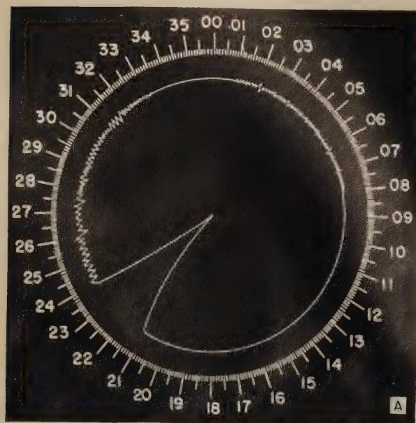
Figure 181. Indicator patterns showing poor brush and slip ring contact.
