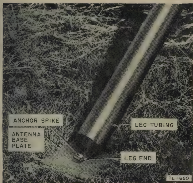
Figure 66. Antenna leg anchored through base plate.
