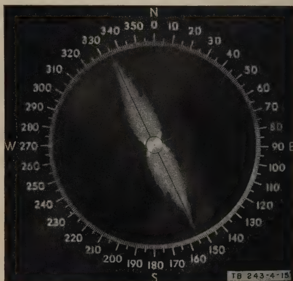
Figure 198. Bearing pattern, showing noisy signal.
