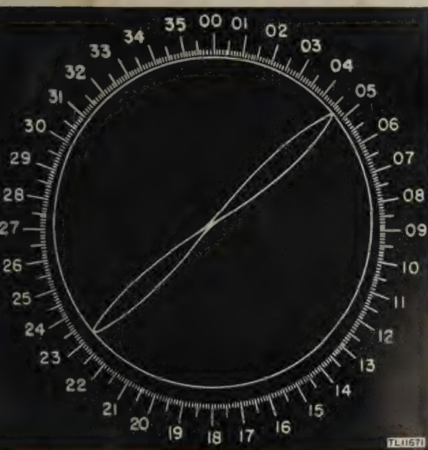
Figure 107. Bearing indicator pattern, keyed c-w signal.
