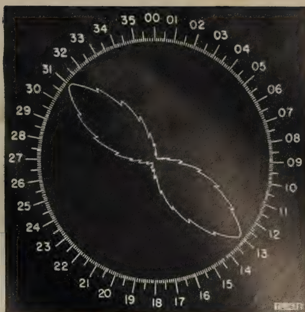
Figure 108. Bearing indicator pattern, modulated signal.
