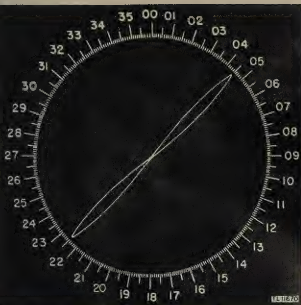
Figure 106. Bearing indicator pattern, strong c-w signal.
