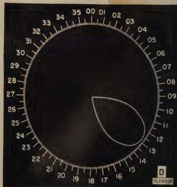
Figure 105. Variations of sense pattern with SENSE GAIN.
