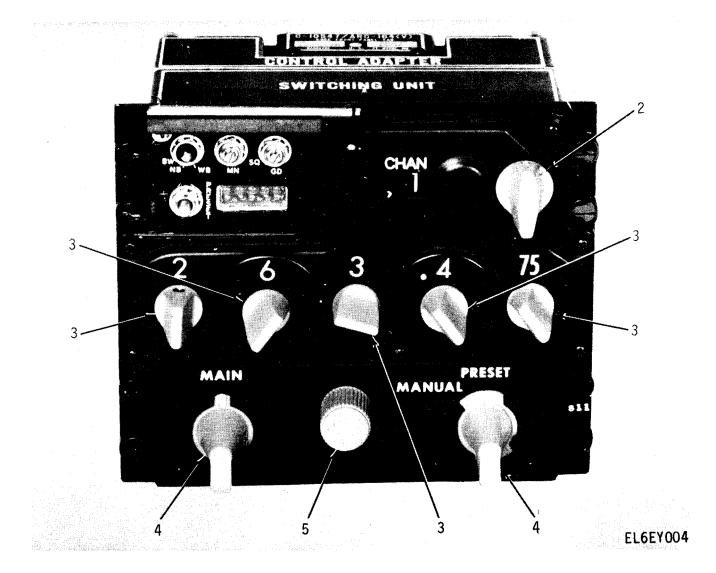
Figure 3. Switching Unit (1A1).
