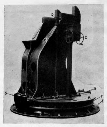
FIGURE 169.-Racer-pedestal assembly.
