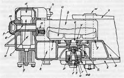
FIGURE 93 .- Bottom carriage, assembled view, firing position.
