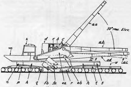
FIGURE 107 .- 14-inch railway mount, M1920.
