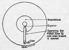
FIGURE 31.-Automatic ejection of primer, firing lock, Mk. I.
