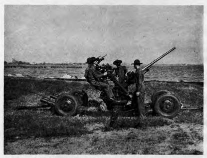
FIGURE 200 .- 37-mm automatic cannon on trailer mount in firing position.
