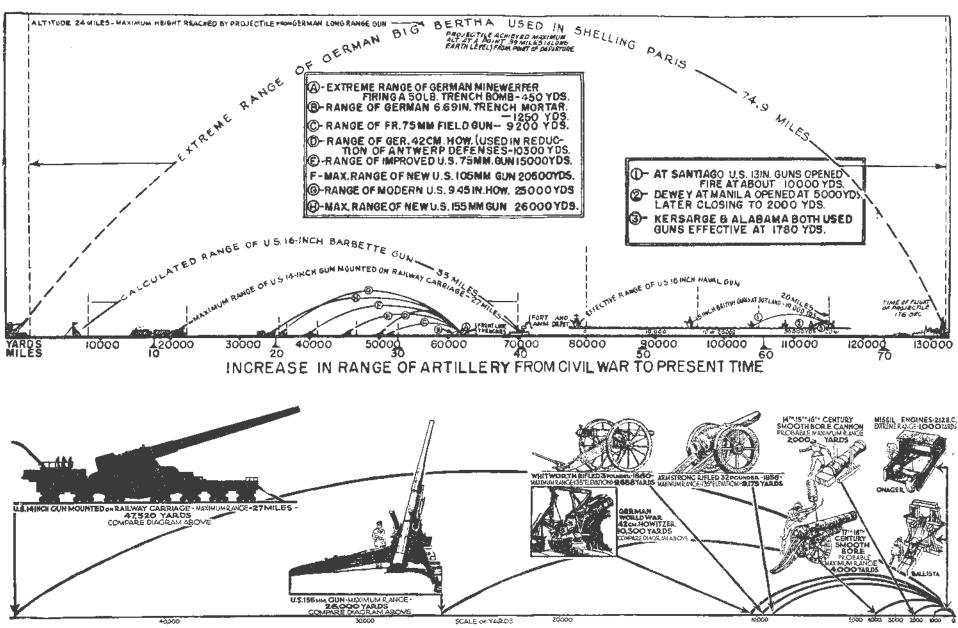
Examples of artillery typical of their times, and their respective ranges, from the ancient missil engines of 212 B. C. to the 42-contimeter German howitzers used at Antwerp in the World war, as compared with examples of America's most moderns guns, maximum ranges of which are in excess of comparative weapons employed in the World war.
