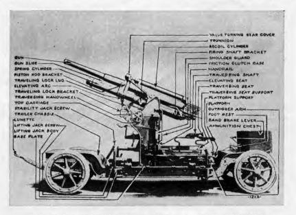
is taken off the disks and the carriage can be traversed freely by pulling or pushing the platforms. The 24 conical rollers on which the top carriage rests and turns are spaced by a bronze distance ring which prevents jamming and insures a proper distribution of the load.
