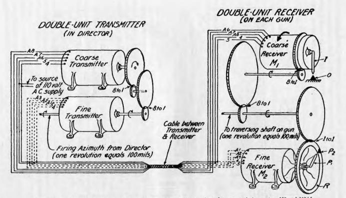
FIGURE 179 .- Schematic diagram of double-unit azimuth transmitter-receiver, data transmission system M2 and M2A1.
