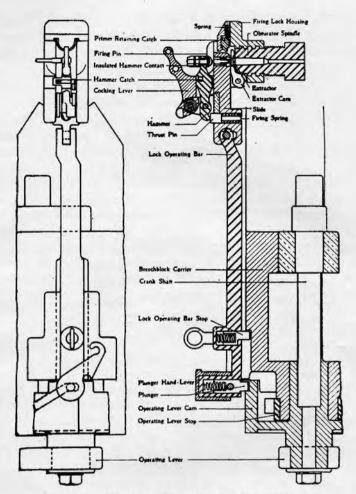
FIGURE 30 .- Firing lock, Mk. I, and operating mechanism.
