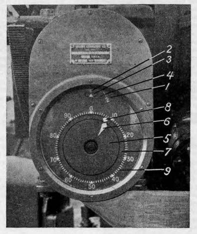
FIGURE 180 .- Elevation receiver,
