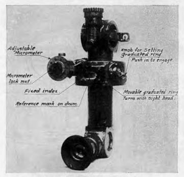
FIGURE 91.-Panoramic telescope, M2.
