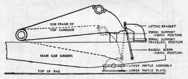
FIGURE 108 .- Top carriage lifting mechanism.
