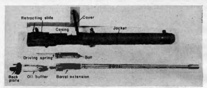
FIGURE 191.-Principal parts of caliber .50 machine gun, M2.
