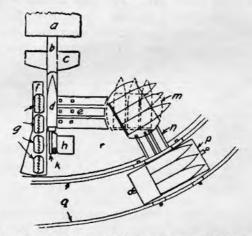
FIGURE 78 .- Loading mechanism, 16-inch barbette carriage.
