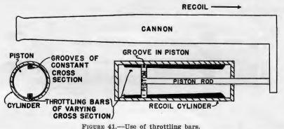
FIGURE 41. Use of throtting bars.
