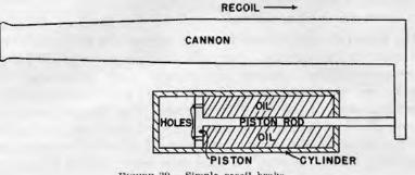
FIGURE 39.-Simple recoil brake.
