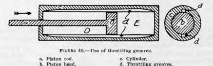
during recoil could be controlled. Another method was devised which provided orifice control through the use of throttling bars (see fig. 41) attached to the cylinder walls and operating in grooves of constant cross-section cut in the piston. Throttling grooves are used in practically all modern recoil mechanisms employing this general type of orifice control.
