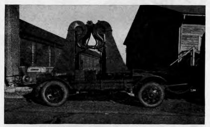
FIGURE 132 .- M1A1 sound locator in traveling position.
