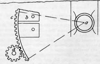
FIGURE 58 .- Elevating rack mechanism.
