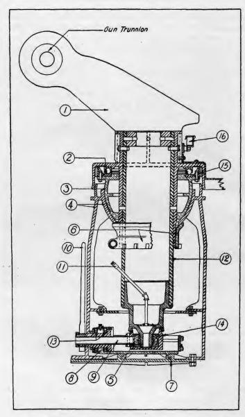
FIGURE 163.-Top carriage pedestal and leveling mechanism.
