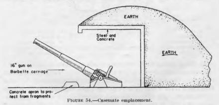
that the gun and crew are protected except from the immediate front. This structure of course limits the field of fire to something less than 180°, although permitting the maximum angle of elevation. Power plant, ammunition storage and service, and plotting room are all bombproofed. The battery is almost as difficult to gasproof
