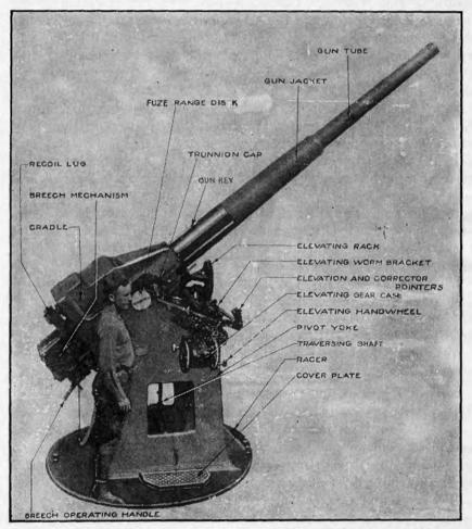
FIGURE 152 .--- 3-inch antiaircraft gun, M1917A2 and mount, M1917 (right side).
