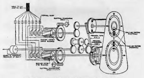
FIGURE 171 .- Azimuth indicator data transmission system, M4.
