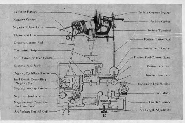
FIGURE 128 .- Schematic diagram of the lamp mechanism and control box.
