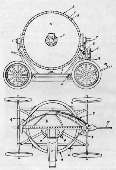
FIGURE 148 .- 60-inch open-type searchlight with high-intensity lamp.
