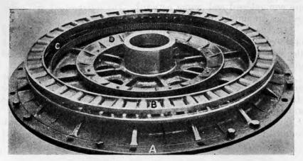
FIGURE 168.—Base plate—roller assembly.
