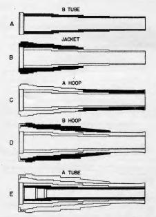
FIGURE 6.-Order of assembly, built-up cannon, 16-inch howitzer, M1920.
