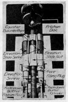
FIGURE 59.—Elevating friction device, 12inch disappearing carriages, M1897 and M1901.
