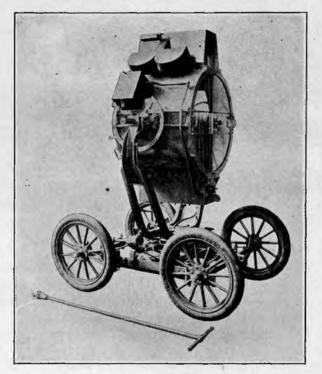
FIGURE 146 .- 36-inch barrel-type searchlight.
