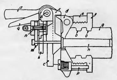
FIGURE 28.-Firing mechanism, seacoast, M1903.
