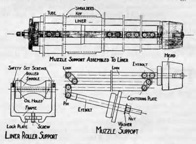
FIGURE 151.-Liner and equipment for inserting and removing.
