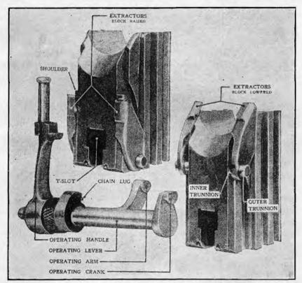
FIGURE 23.-Breechblock and operating lever, 3-inch AA gun, M1917.
