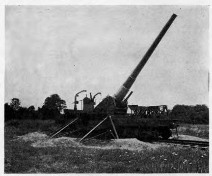
FIGURE 101.-S-inch railway gun mount, M1.
