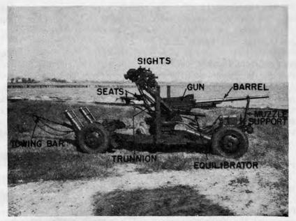
FIGURE 201.-37-mm automatic cannon in traveling position.
