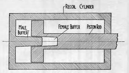
FIGURE 47.-Counterrecoil buffer (simplest type).
