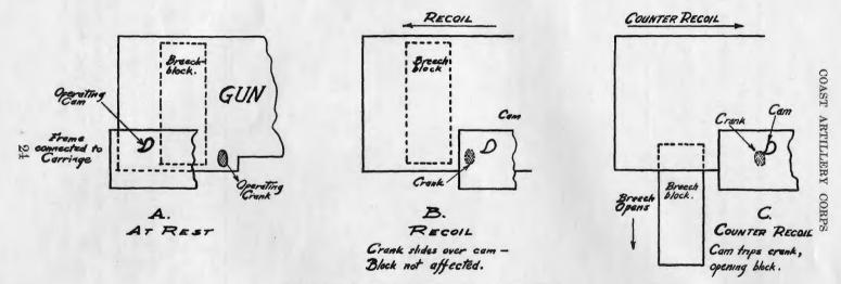
FIGURE 24.-Operation of opening AA gun breechblock.
