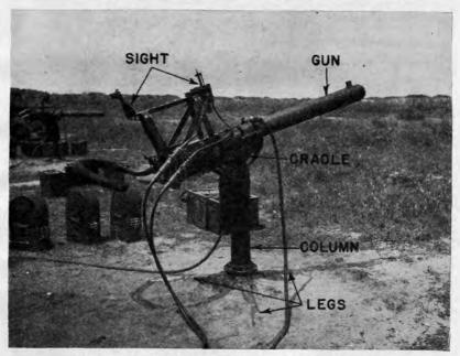
FIGURE 190.-Caliber .50 machine gun, M2, on mount, M2.
