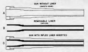
FIGURE 10 .- Cold-worked gun with removable liner, 3-inch, callber .50 AA gun.
