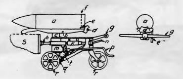
FIGURE 70.-Ammunition loading truck.
