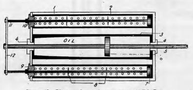
FIGURE 68.-Diagram of separate type counterrecoil buffer.
