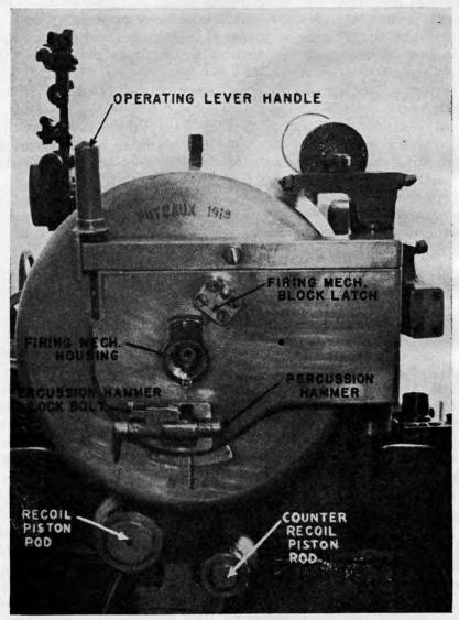
FIGURE 34.-155-mm breechblock showing firing mechanism housing.
