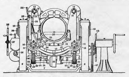
FIGURE 84.-12-inch mortar carriage, M1908 (rear elevation).
