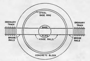
FIGURE 110.—Permanent emplacement for 14-inch railway mount.
