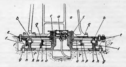
FIGURE 153 .- Base plate and racer assembly.
