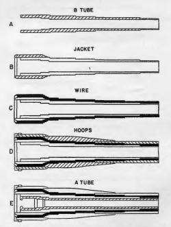
FIGURE 7.-Order of assembly, wire-wrapped cannon, 16-inch gun, M1919.
