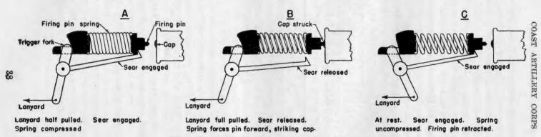
FIGURE 37 .- Operation of continuous pull firing mechanism.
