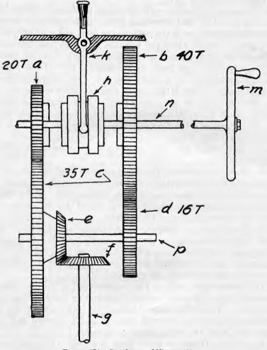
FIGURE 154.-Speed gear shift assembly.
