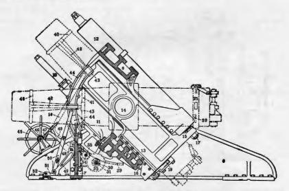
FIGURE 83.-12-inch mortar carriage, M1908 (longitudinal section).
