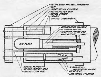
FIGURE 77.-Schematic diagram of recoil system, 16-inch barbette carriage, M1919.
