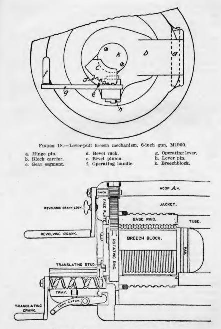
FIGURE 19 .--- Diagram translating roller mechanism.
