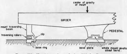
FIGURE 111.-Mount traversing mechanism, 14-inch railway gun.
