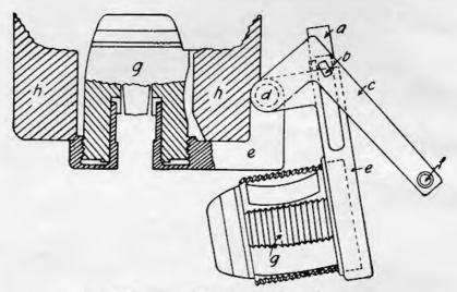
FIGURE 17 .- Lever-pull breech mechanism, 155-mm gun.
