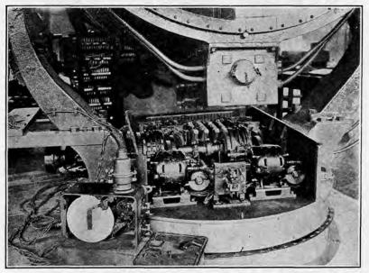
FIGURE 123.-Synchronous-relay, distant electric control, mounted on harbor defense searchlight.
