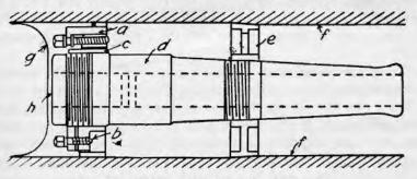
FIGURE 12 .- 2.95-inch (18-pounder) subcaliber tube.
