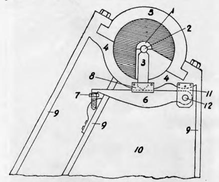
FIGURE 103 .- Antifriction device, 12-inch railway mortars.
