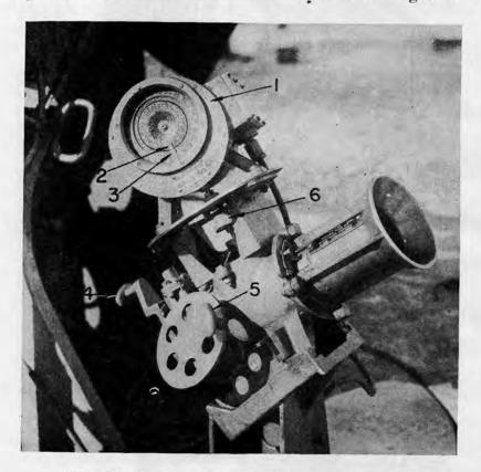
FIGURE 187.-Continuous fuze setter, M3, and fuze range receiver.
