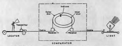
FIGURE 138.-Diagram showing connections of light and locator to comparator.
