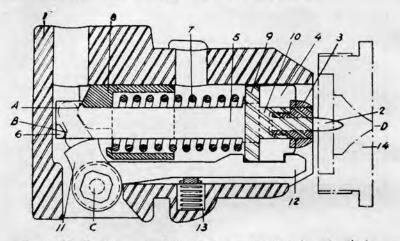
FIGURE 36 .- Continuous pull firing mechanism, new type (top elevation).
