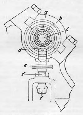
FIGURE 156.—Antifriction device assembly.
