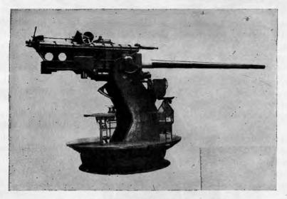
FIGURE 167 .- 105-mm antiaircraft gun mount, M1.
