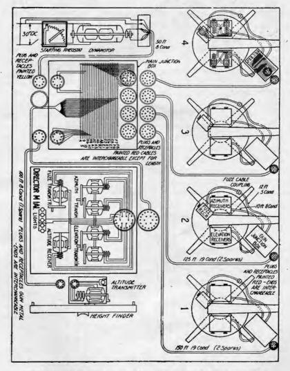
FIGURE 178.-Schematic diagram self-synchronous transmission system, M2.
