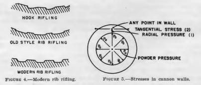
8. Manufacture.—a. (1) If we take a cross-section of a cannon (fig. 5) and imagine a powder pressure acting at right angles to the bore, we find that there are two stresses set up. One is a radial compressive stress, acting outward (1). The other, and the greater test of the strength of the cannon, is the tangential stress (2)—a tension tending to rupture the walls of the gun. There is also a longitudinal stress tending to elongate the cannon.
