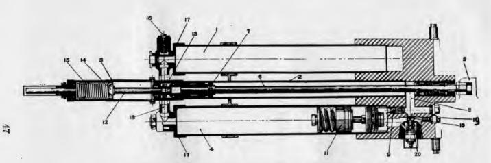
FIGURE 51 .--- Recoil system, 3-inch antiaircraft mount, M2 (top elevation).
