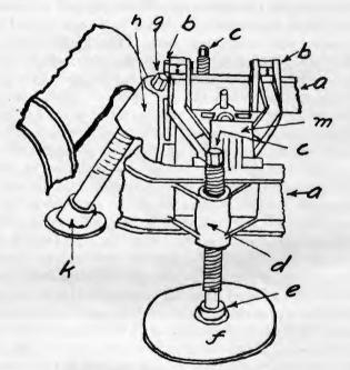
FIGURE 159 .- Stability and lifting jacks.
