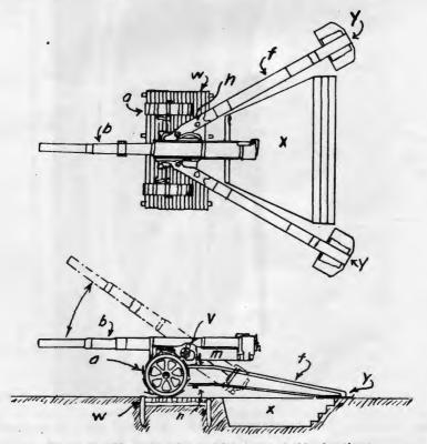
FIGURE 85 .- Mount in firing position (top and side elevations).
