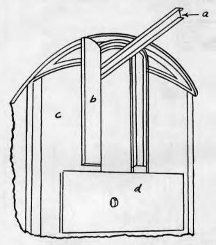
FIGURE 114.—Ammunition car, end sketch. a. Rail trolley extension. b. End door. c. Car end. d. Hinged floor plate.
