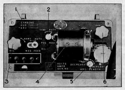
FIGURE 129.-Exterior of lamp control box.
