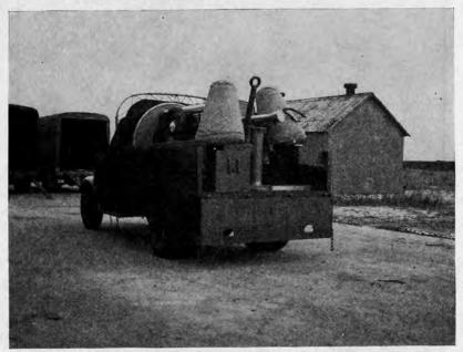
FIGURE 134 .-- M2 sound locator in traveling position (parts loaded into cargo truck).
