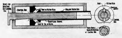
FIGURE 43.-Operation of control rod.
