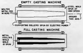
FIGURE 9.-Centrifugal casting.
