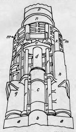
FIGURE 76 .- Top view of recoil and recuperator systems, 16-inch barbette carriage, M1919.
