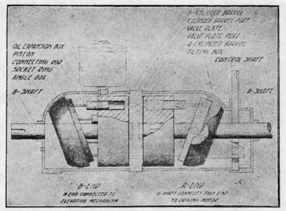
FIGURE 61 .- Diagrammatic sketch of Waterbury hydraulic speed gear.
