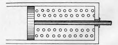
FIGURE 44 .- Cross-sectional diagram showing use of two concentric springs.
