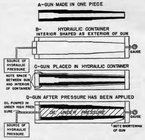
FIGURE 8.-Cold-work process (container method).
