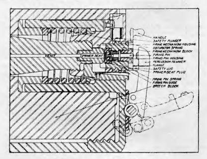
FIGURE 35 .- 155-mm percussion-type firing mechanism.
