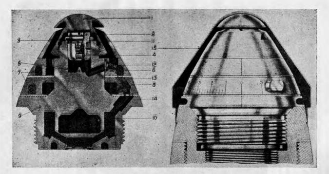
FIGURE 186 .- Antiaircraft time fuze, Mk. III.
