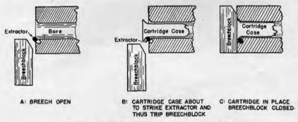
FIGURE 25 .- Automatic closing of AA breechblock.
