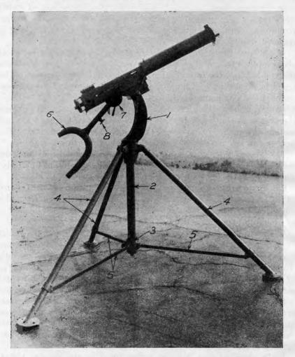
FIGURE 198.—Browning machine gun, caliber .50, M1921, and AA machine gun tripod mount, M1.
