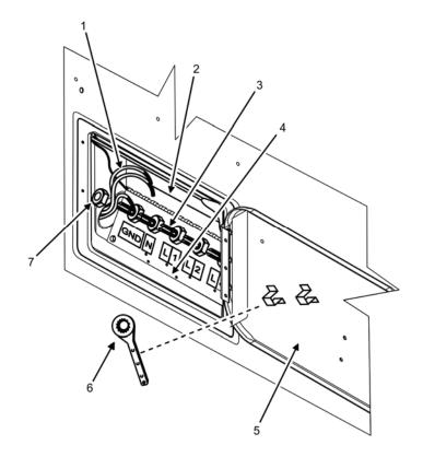
Figure 6. Installation of Load and Ground Cables.
