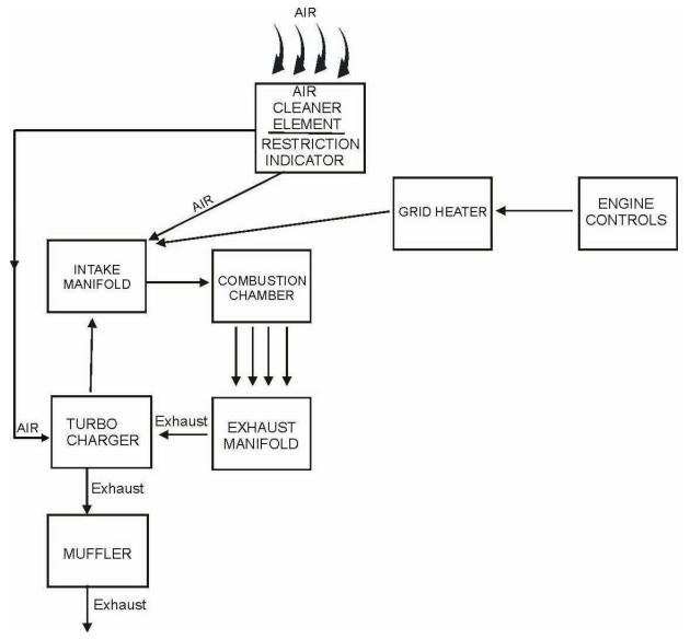
Figure 6. Air Intake and Exhaust System.
