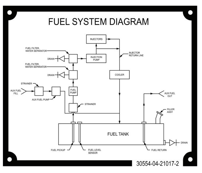
Figure 46. Label, Fuel Diagram — Model 1070/1071.
