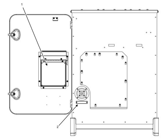
Figure 31. Decal and Instructions Plates, Front — Model 1070/1071.
