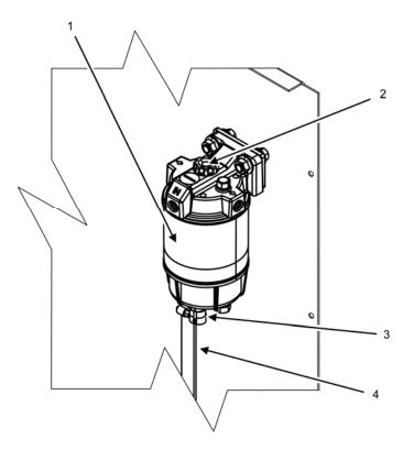
Figure 3. Fuel Filter/Water Separator.
