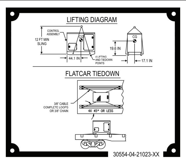
Figure 35. Label, Lifting and Tie Down — Model 1070/1071.
