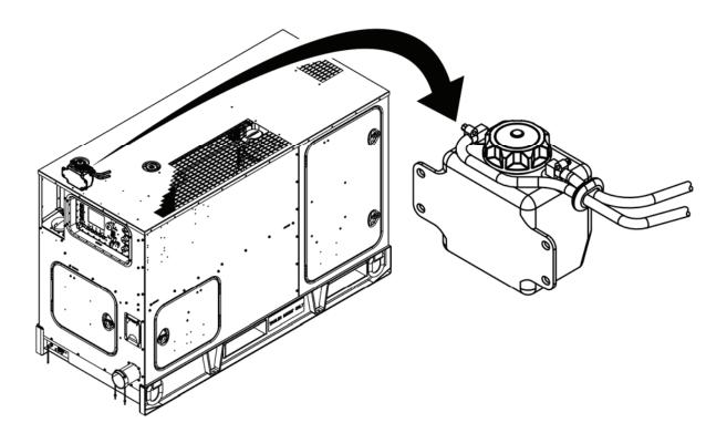
Figure 1. Coolant Overflow Bottle — Location.
