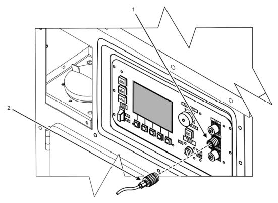
Figure 24. Operator Display Panel — Remote Connection.
