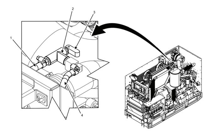
Figure 6. Pressure Relief Valve.
