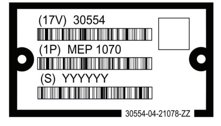
Figure 36. Plate, IUID Identification — Model 1070.
