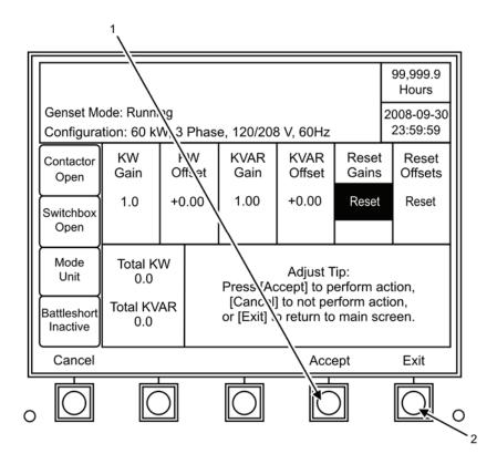
Figure 10. Parallel Adjustment Screen, F.
