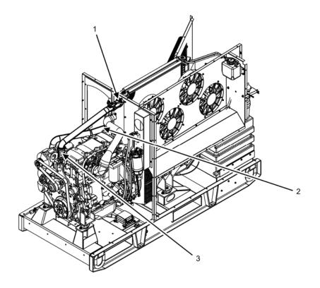
Inspect Radiator Hoses, Interconnecting Tubes, and Clamps
