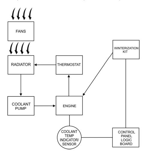
Figure 4. Engine Cooling System.
