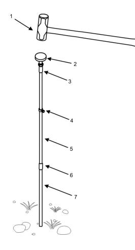
Figure 4. Install Ground Rod With Sledge Hammer.
