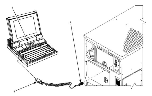
Figure 25. Remote PC — Connection.
