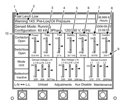
Figure 19. Main Control Screen Status Indicators 120/208 V 3 Phase.
