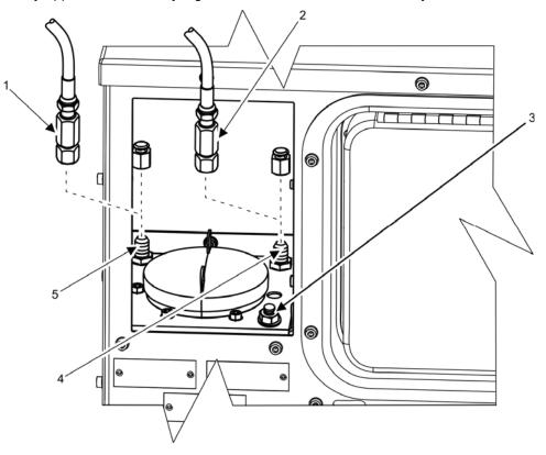
Figure 5. Auxiliary Fuel Supply Connections.
