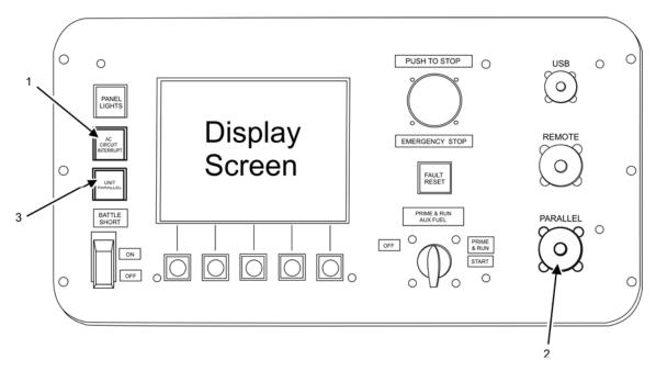
Figure 12. DCS Panel, Remove From Parallel.
