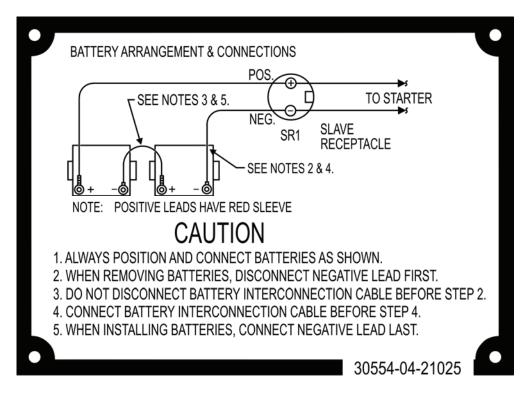
Figure 50. Plate, Battery Connection — Model 1070/1071.
