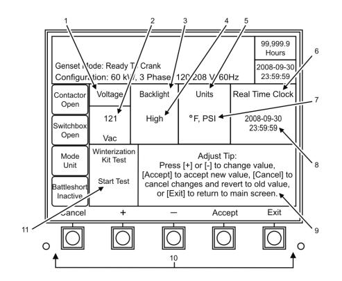
Figure 10. [Adjustments] Screen 1 — Adjust.
