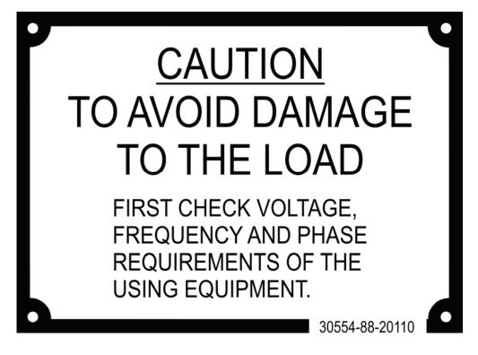
Figure 51. Label, Caution, Voltage Connection — Model 1070/1071.
