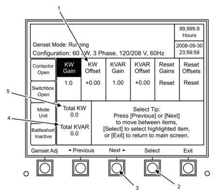
Figure 5. Parallel Adjustment Screen, A.
