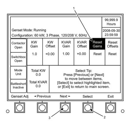
Figure 9. Parallel Adjustment Screen, E.
