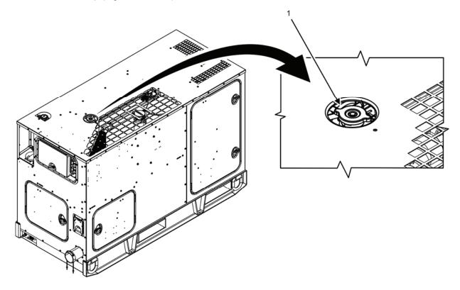
Figure 4. Radiator Fill — Exterior.
