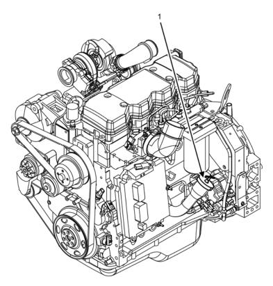
Figure 2. Oil Service Detail — Left Side.
