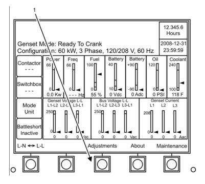
Figure 14. Main Screen Showing Adjustments — Location.
