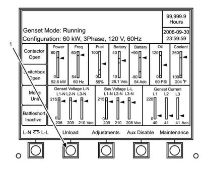
Figure 11. Soft Unload Key.
