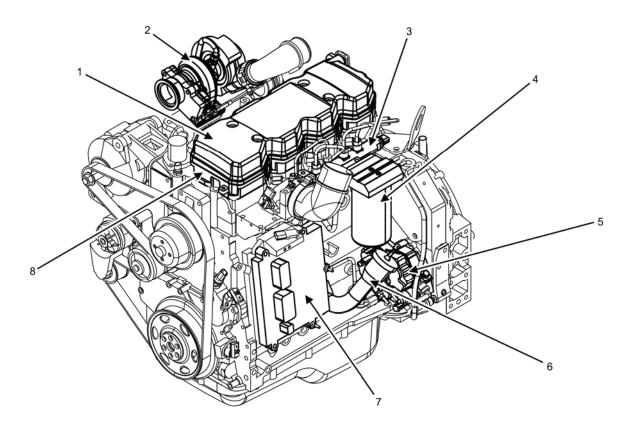
Figure 5. Engine Components — Left Side.
