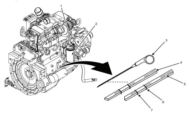
Figure 1. Oil Service Detail — Right Side.
