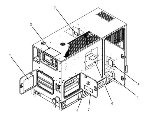
Figure 30. Decal and Instructions Plates, Top and Inside — Model 1070/1071.
