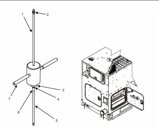
Figure 3. Install Ground Rod With Slide Hammer.
