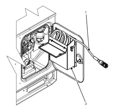
Figure 1. Storage Box and Cable — Location.
