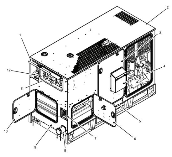
Figure 2. Rear and Right-Side View with Doors Open.
