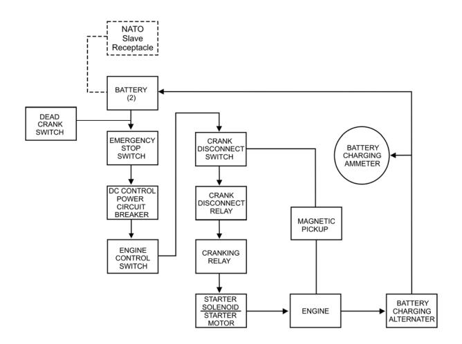
Figure 2. Engine Starting System.
