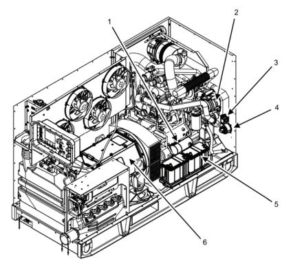
Figure 9. 24-VDC Electrical and AC Generator Components — Right Side.
