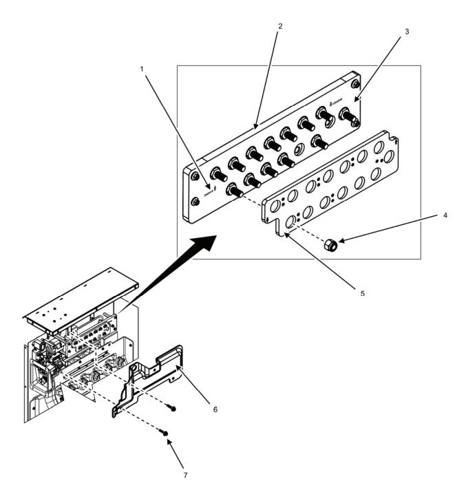
Figure 8. Configure Voltage Selection Board.
