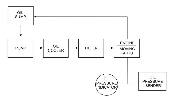
Figure 5. Engine Lubrication System.
