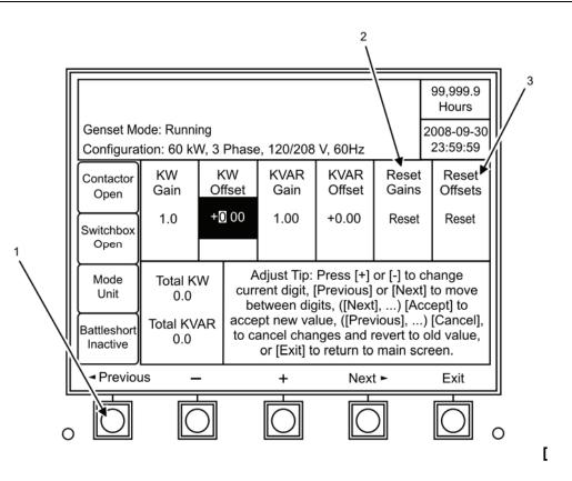
Figure 7. Parallel Adjustment Screen, C.
