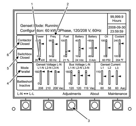
The DCS panel may briefly display an initializing screen with all data grayed out before the main display screen appears.
