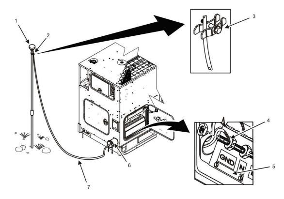
Figure 2. Grounding Connections.
