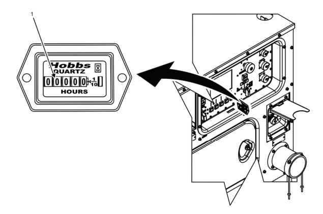
Figure 17. Generator Hour Meter.
