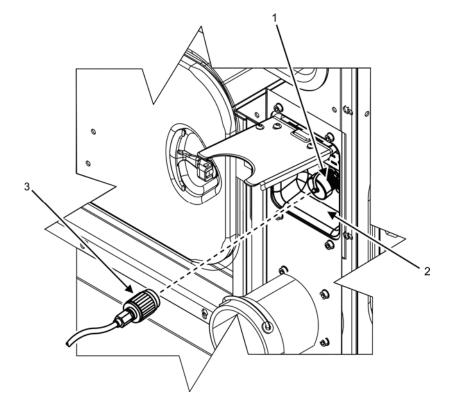
Figure 3. Switch Box Paralleling Receptacle.
