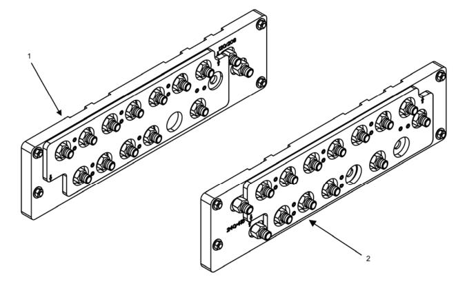
Figure 7. Voltage Selection Board.
