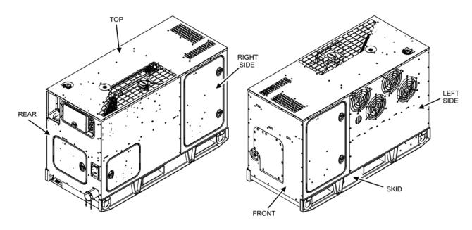
Figure 1. Skid-Mounted 60 kW AMMPS Generator Set.
