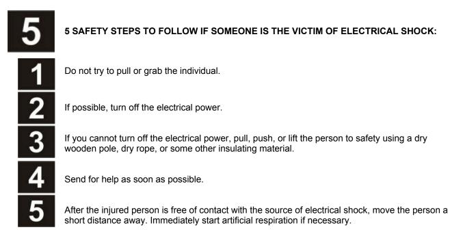
The Warning Summary summarizes critical safety and hazardous material warnings that must be understood and applied during operation and maintenance of the Advanced Medium Mobile Power Sources (AMMPS) generator sets.
