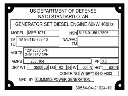
Figure 34. Plate, Identification — Model 1071.
