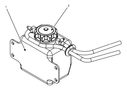
Figure 2. Coolant Recovery Assembly.
