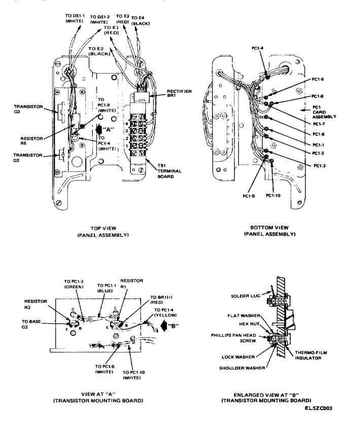
Figure 8.1, Parts locations, generator unit panel assembly, G-77/G.
