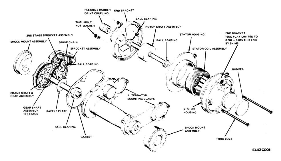
Figure 11-1. Disassembly for lubrication (G-77/G).
