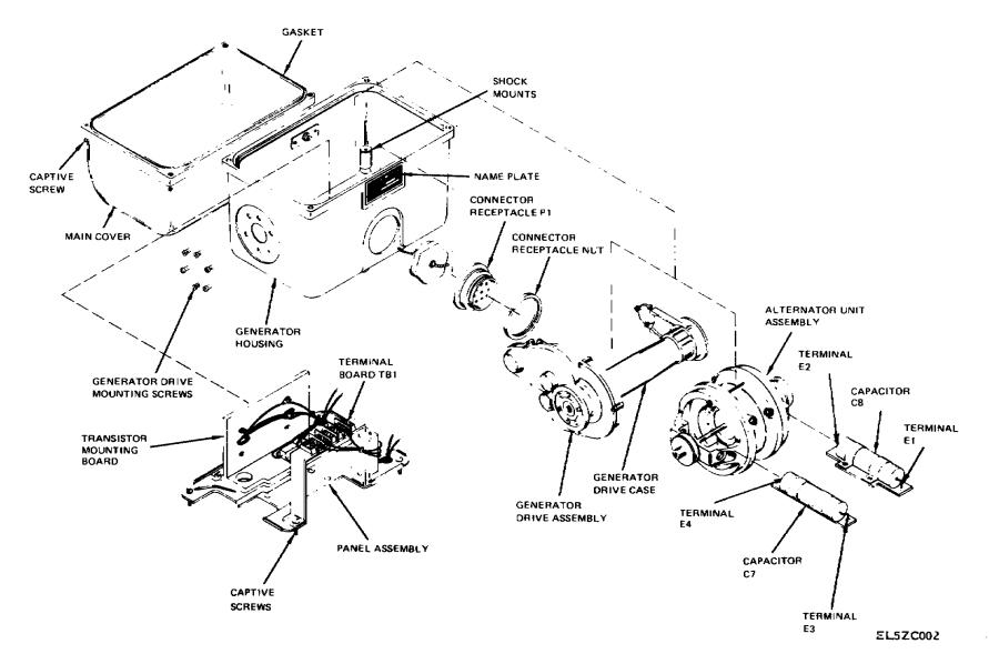
Figure 7.1. Disassembly of housing components (G-77/G).
