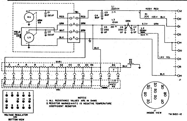
Figure 9. Main schematic diagram.
