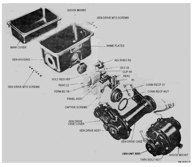
Figure 7. Disassembly of housing components.
