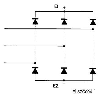
Figure 8.2. Rectifier schematic diagram
