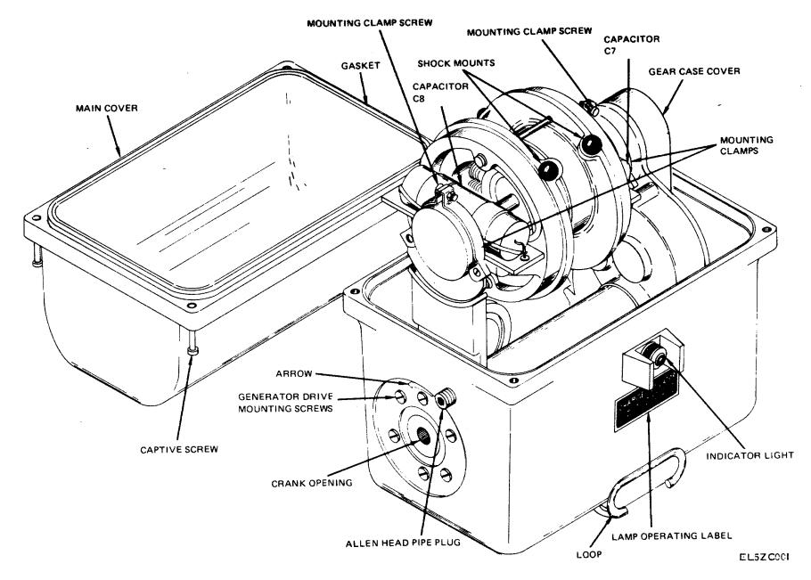
Figure 6.1. Generator unit, main cover removed (G-77/G).
