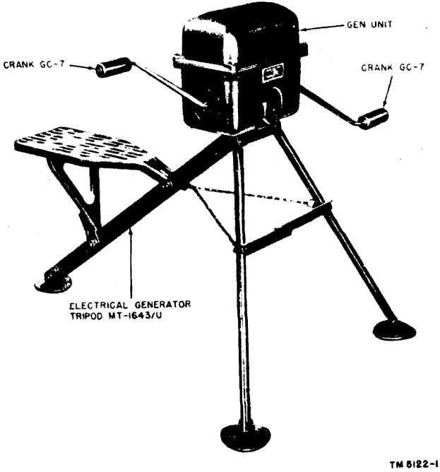
Figure 1. Direct Current Generator G-43/G, components.
