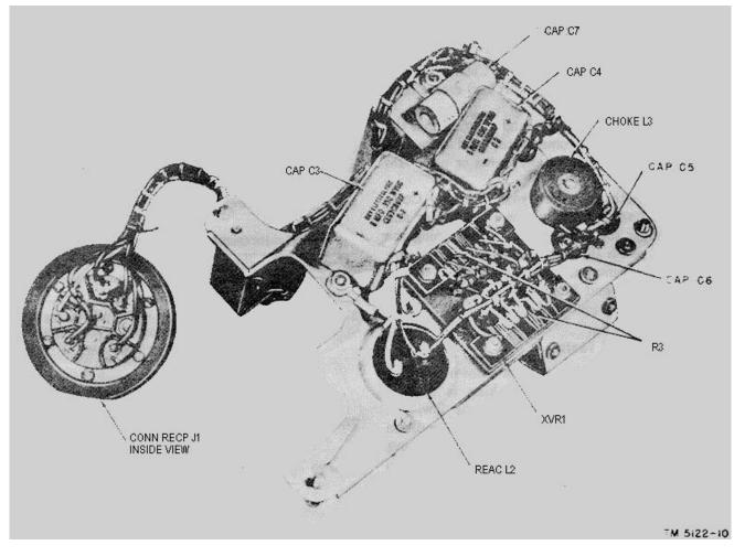
Figure 8. Bottom view of panel assembly.
