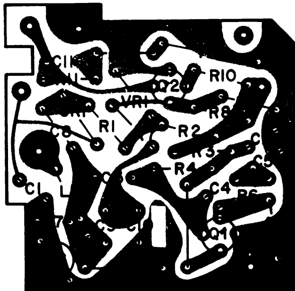
Figure 5-11. Part 17488-3 Local Oscillator (A2A3), Location of Components
