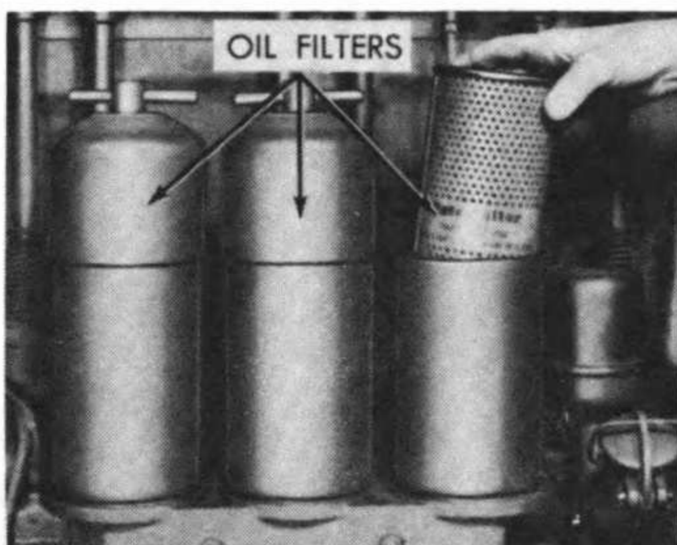
Ref. 17: At each oil change period, wash metallic strainer elements and replace inner filter elements with new elements.
