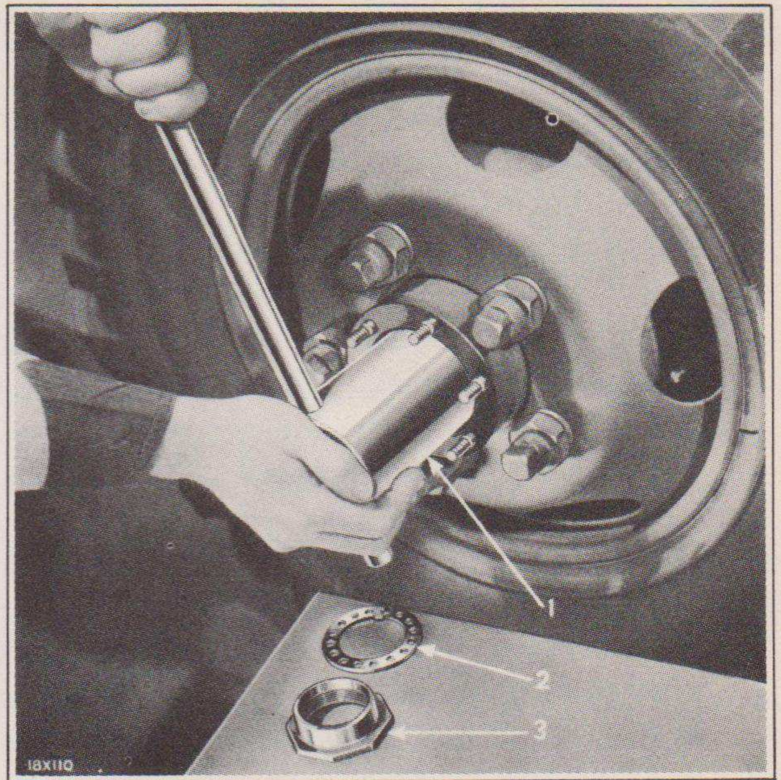
Fig. 48—Removing Rear Wheel Bearing Adjusting Nuts or Adjusting Bearings
