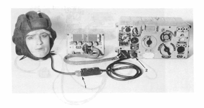
Figure 5-4. Connection of CVC to chest plate switch and radio.
