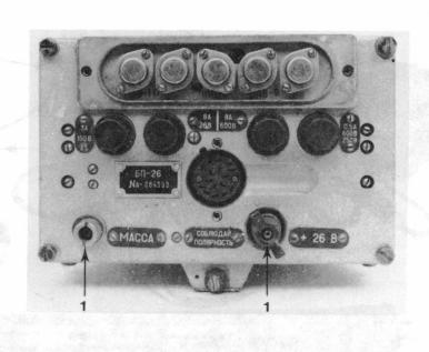
Figure 5-7. Power supply connection points.
