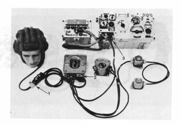
Figure 5-5. Connection of CVC to R-124 and R-124 to R-123M.
