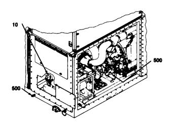
Oil Filter (Disassemble, clean housing, renew element, and reassemble.)(See note 1.) (0)
