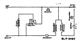
Fig. 28.—Circuit diagram of the Field Artillery telephone, type  $\mathbf{EE} - \mathbf{5}$ .
