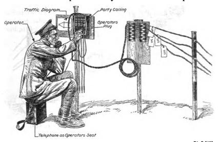
Fig. 10.—Operator answering a call on the monocord switchboard.
