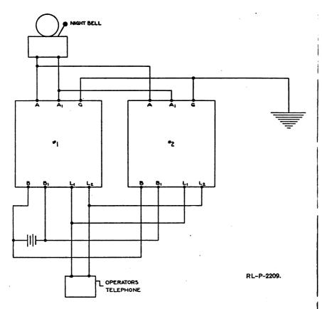
Fig. 29.—Diagram of the connections between two monocord switchboards of type EE - 2 units installed as a single unit.
