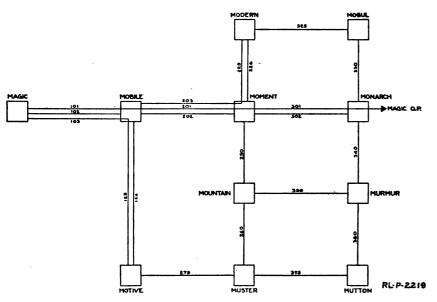
Fig. 36.—Circuit diagram of a division telephone net.
