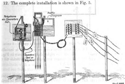
Fig. 5.—A telephone with monocord switchboard of type EE – 2A units with camp telephone as operator's set.
