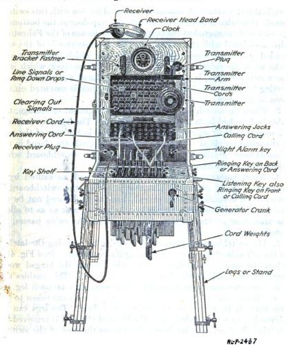
Fig. 40.—A front view of the camp-type switchboard.
