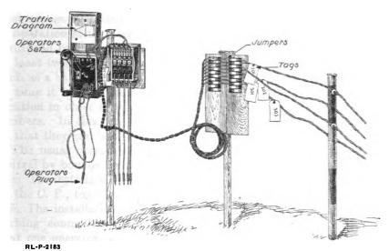
Fig. 8.—Telephone central with monocord switchboard, of type EE - 2 units, using operator's set.
