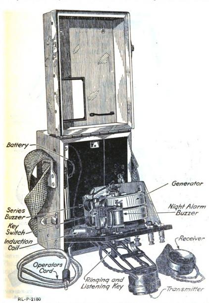
Fig. 32.—View of the interior of a monocord switchboard operator's set, type EE - 64. buzzer, the key switches, and the night-alarm buzzer. The two-bar
