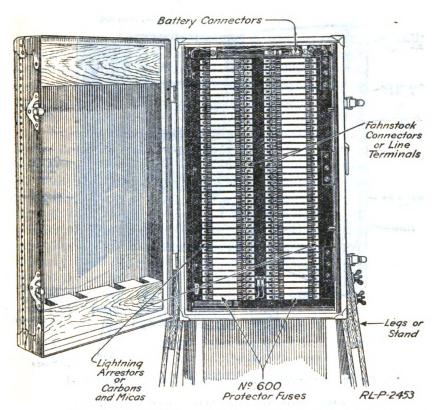
Fig. 41.—The protector panel of the camp-type switchboard.
