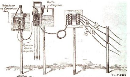
Fig. 5.—A telephone central with monocord switchboard of type EE - 2-A units with camp telephone as operator's set.
