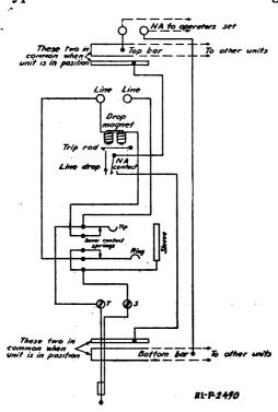
Fig. 31.—Circuit diagram of a type EE - 2-A unit.
