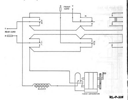
Fig. 45.—A circuit diagram showing the operator calling a subscriber, with the front key in the ringing position, on a camp-type switchboard.
