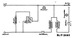
Fig. 28.—Circuit diagram of the Field Artillery telephone, type EE - 5.
