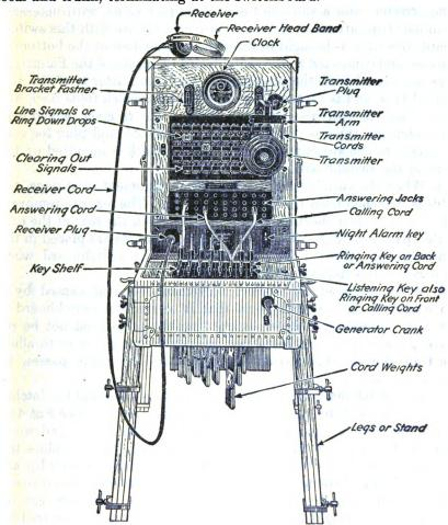
Fig. 40.—A front view of the camp-type switchboard.
