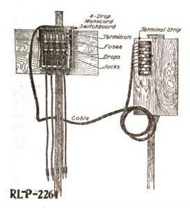
Fig. 2.—Cabling monocord switchboard to a terminal strip.
