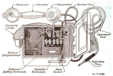
Fig 4.—Camp telephone, type EE - 4, with operator's cord attached.
