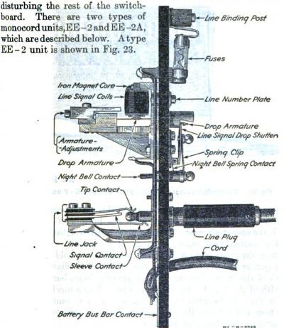
Fig. 23.—Monocord switchboard unit, type EE - 2.
