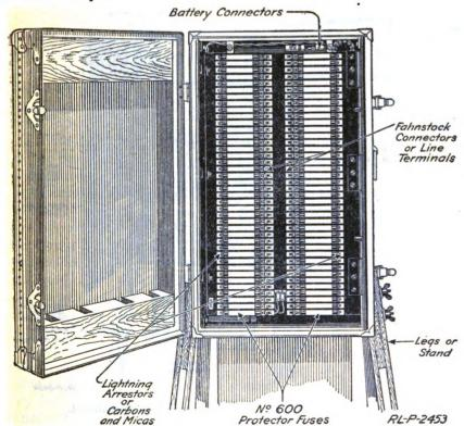
Fig. 41.—The protector panel of the camp-type switchboard.
