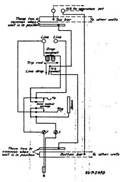
Fig. 31.—Circuit diagram of a type EE - A2 unit.
