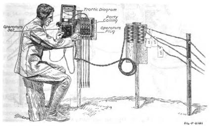
Fig. 11.—Operator preparing to call the called party on a monocord switchboard.
