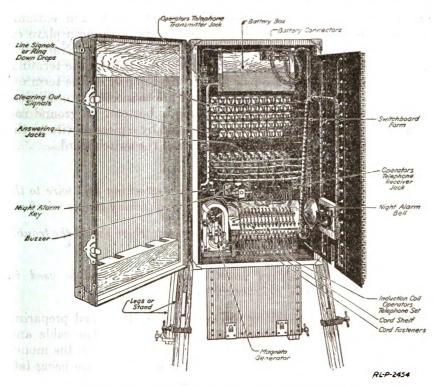
Fig. 20.—Rear view of the interior of the camp-type switchboard.
