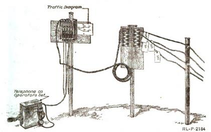
Fig. 3.—Installation of monocord switchboard with a camp telephone for operator's set.
