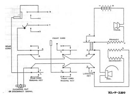
Fig. 44.—A circuit diagram showing the operator answering a call, with the front key in listening position, on a camp-type switchboard.
