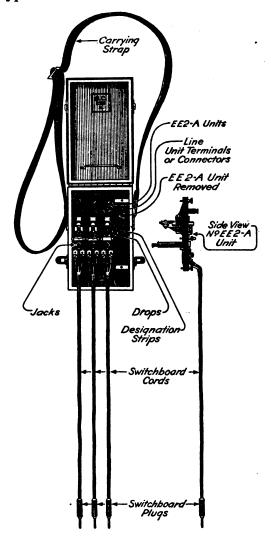
Fig. 30.—Four-line monocord switchboard of type EE - 2-A units.
