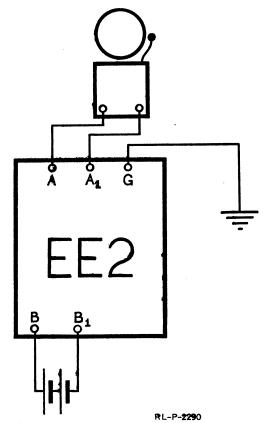
Fig. 6.—Circuit diagram of night alarm with switchboard of type EE - 2 units.
