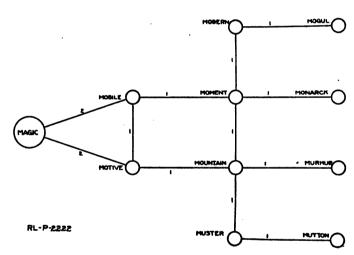
Fig. 39.—Traffic diagram of a division telephone net.
