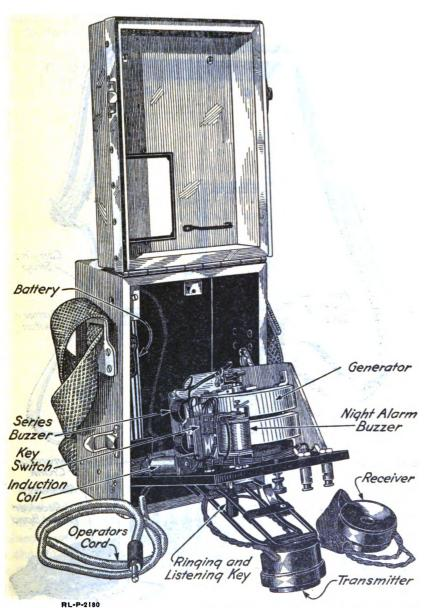
Fig. 32.—View of the interior of a monocord-switchboard operator's set, type EE - 64.
