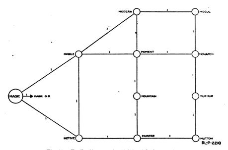
Fig. 38.—Traffic diagram of a division telephone net.
