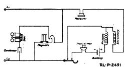
Fig. 27.—Circuit diagram of the camp-type telephone, type EE - 4.
