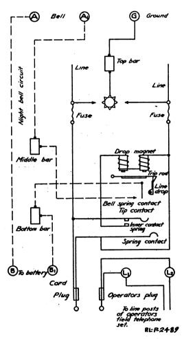
Fig. 26.—Circuit diagram of a type EE - 2 unit.
