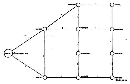
Fig. 38.—Traffic diagram of a division telephone net.
