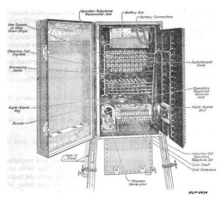
Fig. 20.—Rear view of the interior of the camp-type switchboard.
