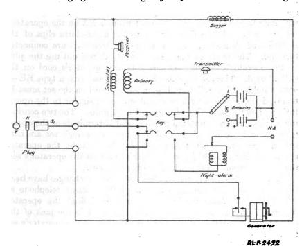
Fig. 34.—Circuit diagram of a monocord-switchboard operator's set, type EE - 64.
