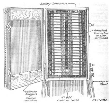
Fig. 19.—The protector panel of the camp-type switchboard.
