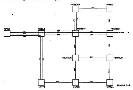
Fig. 36.—Circuit diagram of a division telephone net.
