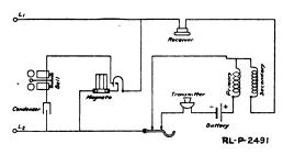
Fig. 27.—Circuit diagram of the camp-type telephone, type EE - 4.
