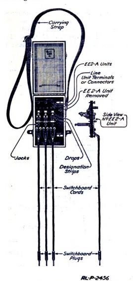
Fig. 30.—Four-line monocord switchboard of type EE - 2A units.
