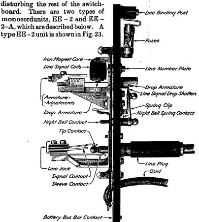
Fig. 23.—Monocord switchboard unit, type EE - 2.
