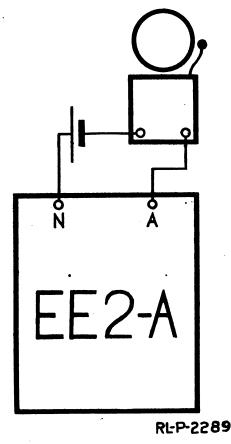
Fig. 7.—Night-alarm circuit with monocord switchboard of type EE - 2A units.
