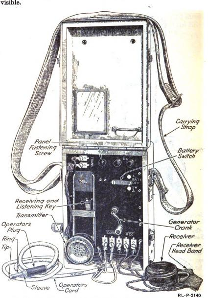
RL-P-2140 Fig. 33.—Front view of a monocord switchboard operator's set, type EE - 64.
