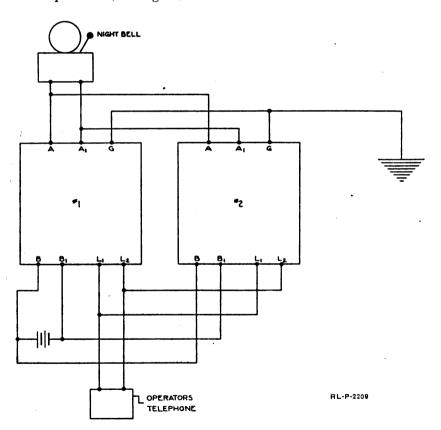
Fig. 9.—A diagram of the connections between two monocord switchboards of type EE-2 units installed as a single unit.
