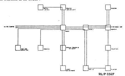
Fig. 9 - IG.—Circuit diagram division telephone net.
