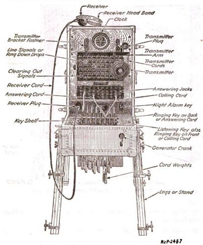
Fig. 18.—Front view of the camp-type switchboard.
