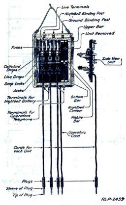
Fig. 25.—Four-line monocord switchboard of type EE - 2 units.
