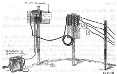
Fig. 3.—Installation of monocord switchboard with a camp telephone for operator's set. strip, installed as in Par. 3, to the left-hand binding posts of the line terminal strip installed as in Par. 4. This connects the drops on the switchboard to the different line circuits.
