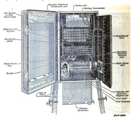
Fig. 42.—A rear view of the interior of a camp-type switchboard.
