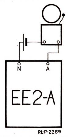
Fig. 7.—Night-alarm circuit with monocord switchboard of type EE - 2-A units.
