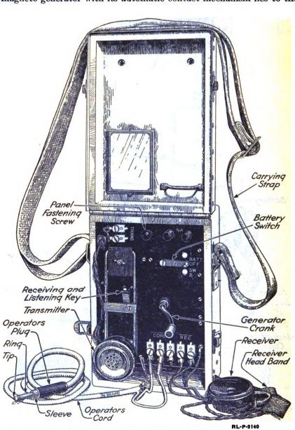
Fig. 33.—Front view of a monocord-switchboard operator's set, type  $\mathbf{EE}$  – 64.
