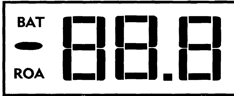
FIGURE 4-1. Active OSM Display Segments.
