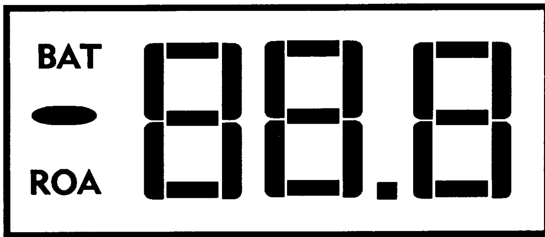
FIGURE 4-4. Active OSM Display Segments.
