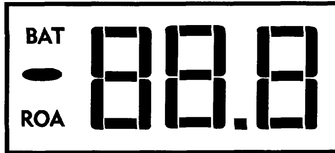
FIGURE 5-5. Active OSM Display Segments.
