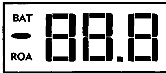
FIGURE 2-1. Active OSM Display Segments.
