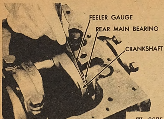
Fig. 104. Checking Crankshaft End Play
