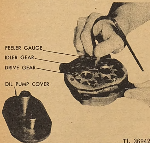
Fig. 290. Checking Oil Pump Gear Clearance to Case
