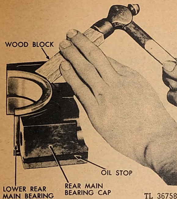
Fig. 106. Removing Main Bearing Shell from Cap
