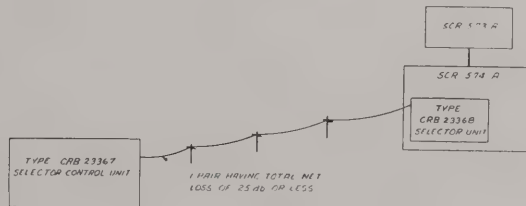
FIGURE 2 — BLOCK DIAGRAM OF CONTROL SYSTEM
