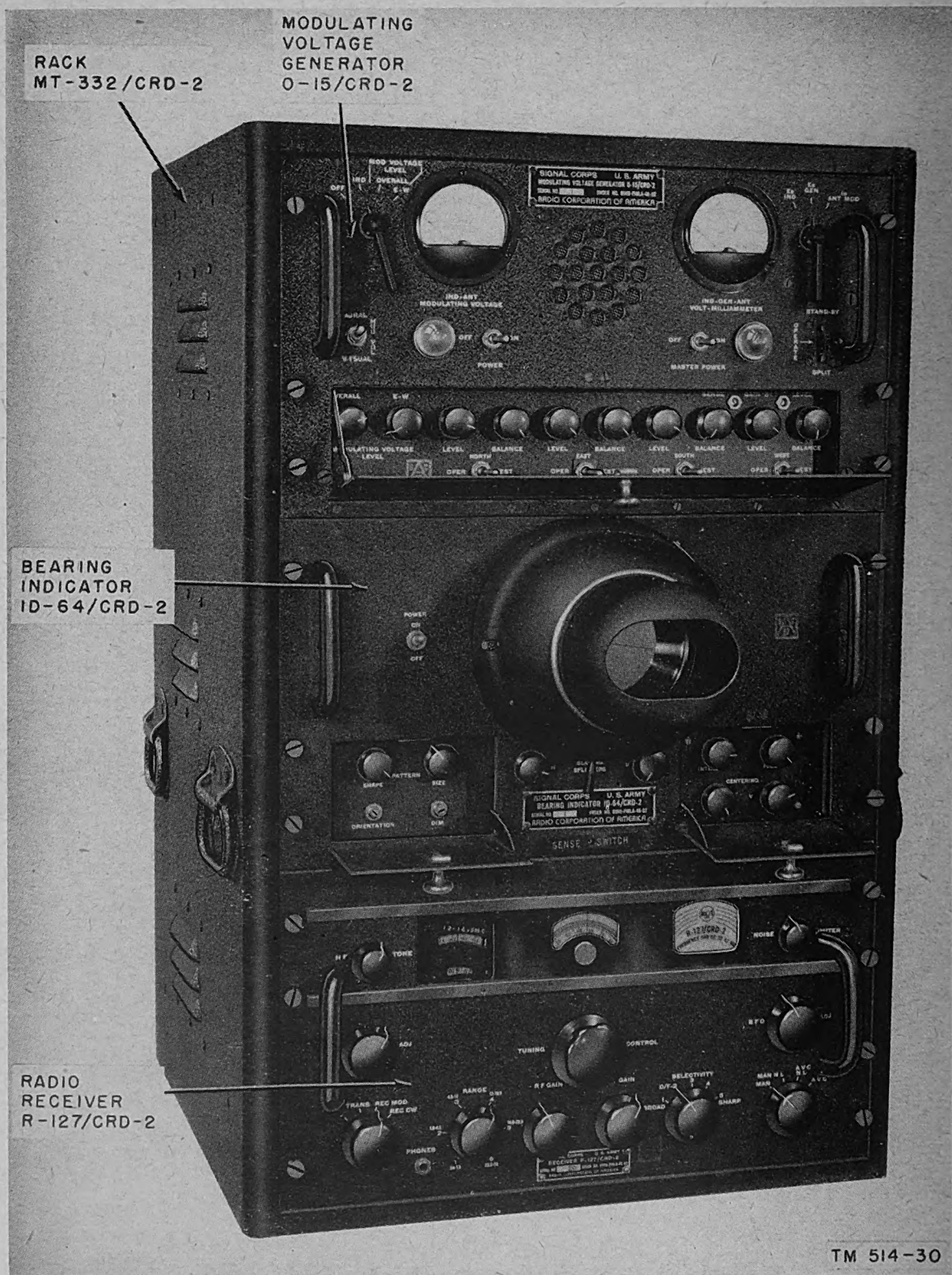
Figure 10. Rack MT-332/CRD-2, components installed.
