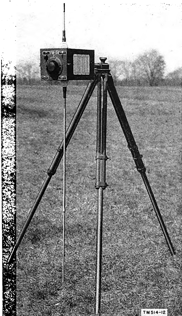
Figure 16. Radio Transmitter BC-1149-A, mounted on tripod.
