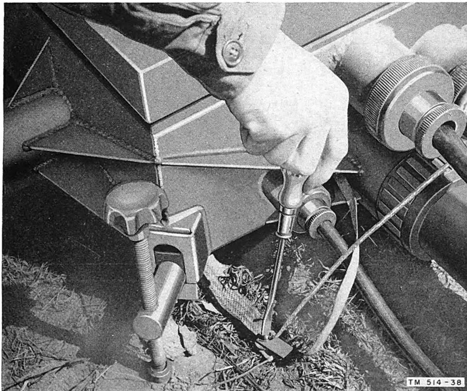
Figure 40. Connecting a ground strap for Junction Box J-96/CRD-2.
